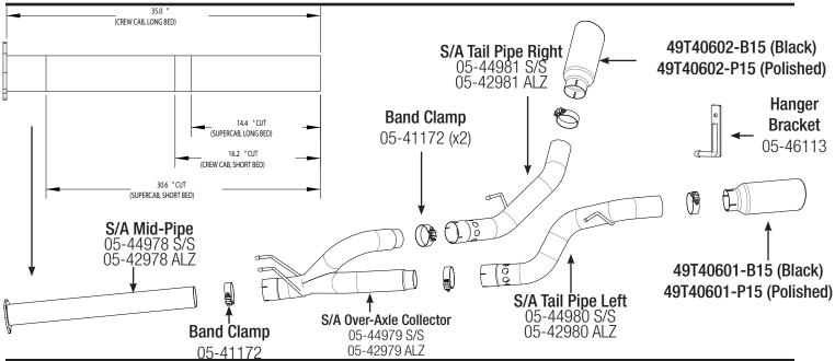
Step 1: (Read Instructions prior to installation) Loosen mounting flange at rear of particulate filter before muffler.
