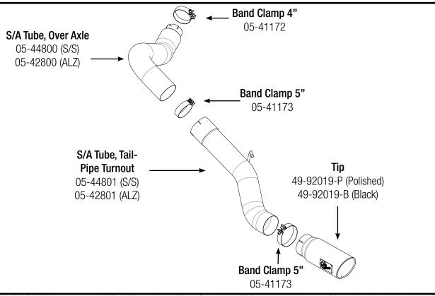
Professional installation is highly recommended. (Read instructions prior to installation) This system requires an aftermarket electronic module, To work properly with the vehicle. Make sure to always have at least (2) stands or jacks on hand to support the removal of OE system. Also for the installation of aFe system. Any Removal of rubber isolation mounts may require using a spray lubricant such as WD40 and a pry bar.
