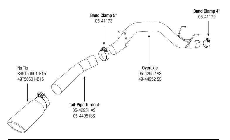
Step 1: (Read Instructions prior to installation) Loosen up clamps (x2), as well as the bolt bracket (x1) holding down the sensor bung wire. save bolt it will be re-used, (when installing new aFe exhaust)
