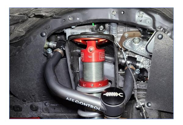
Insert the ball joint stud into the upright and install the castle nut using a 26mm socket. Tighten to 80 ft  $\cdot$  lbs and continue to tighten until the castle slots lines up with the next cotter pin hole.
