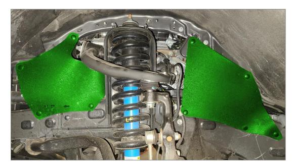
Unbolt the brake line brackets from the inner fender with a 10mm socket and the junction on the rail with a 12mm socket. This will give room for the cross bolt to be removed/installed.
