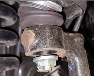
4 Use a hammer and hit the upright as shown below. The ball joint tapered stud should pop loose after 4-5 hits. If the stud is being stubborn and does not want to break loose, you can use a ball joint puller tool. Using the puller in conjunction with a couple of smacks with the hammer should pop it loose.
