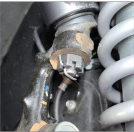
Slide the OE rubber sleeve on the ABS line so it lines up with the tab on the UCA and use the provided zip tie to secure the ABS line to the arm.
