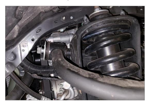
Cut the bolt head off and slide the bolt towards the back to remove.
