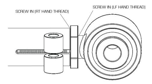
Next adjust just the double adjuster out until the gap between the control arm and the adjuster is approximately 0.220"- 0.250".
