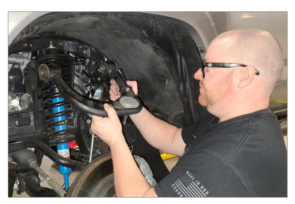
The aFe Control UCA's are neutrally adjusted from our factory. However, if the bushing ends look like they are not even or have been mistakenly unscrewed, you can zero-base the arms to get back to neutral adjustment. First step is to screw-in both the adjuster and bushing end into arm making them as short as possible.
