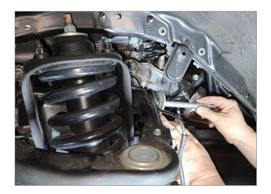
Finally, remove the loose castle nut and control arm should be free to remove from the vehicle.
