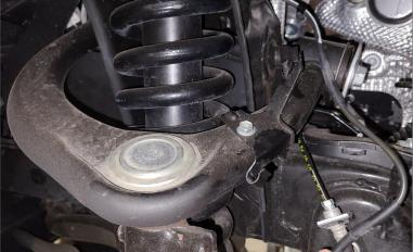
Remove the factory cotter pin using a pick. Loosen but do not remove the castle nut. Leave about a  $\frac{1}{4}$ " of gap between the upright mount and nut.
