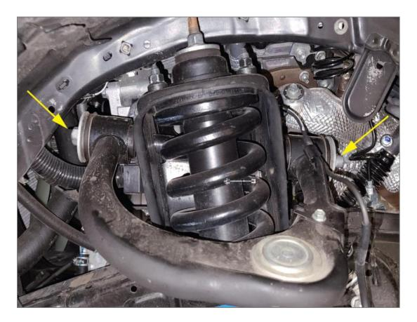
Pull the bolt forward so you are in a good position to use the saw on the bolt. Note: Inner corrosion may make this difficult to slide.
