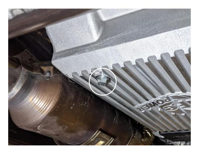
20. Hold the transmission pan up into position, aligning the bolt holes. Install one (1) M6x1.0x20 socket head screw and M6 washer into each of the four (4) corners to hold the pan into place.
