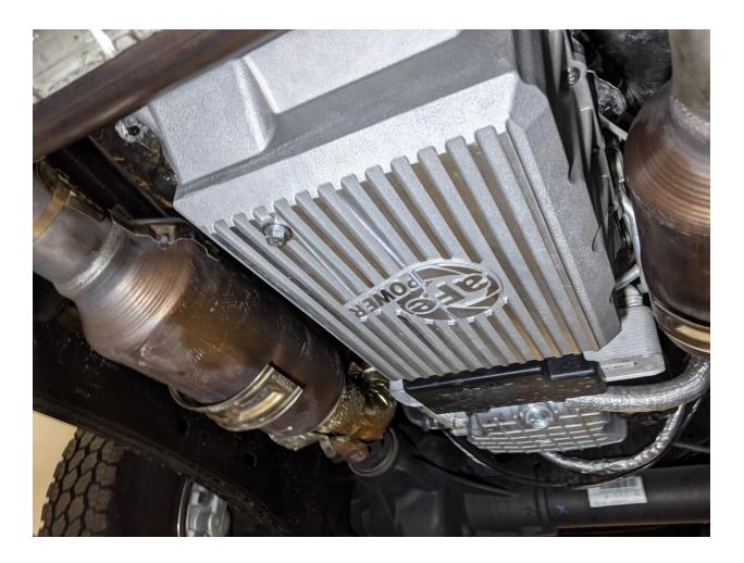
29. Once again with the vehicle running in park, remove the fluid level plug. Either allow the excess fluid to drain or add fluid until it is even with the bottom of the level port.
