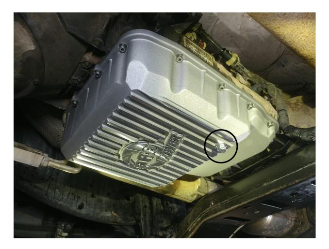
18. Install the supplied M12x1.25 magnetic drain plug and M12 crush washer into the bottom drain hole.
