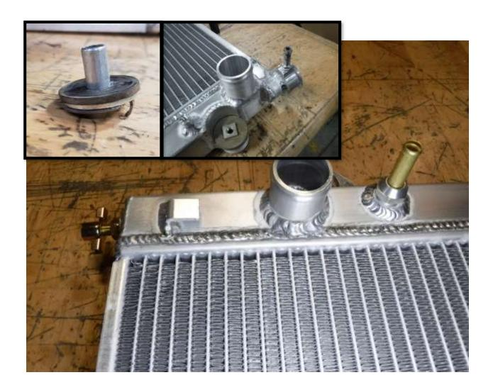
16. Install the two (2) supplied transmission fittings onto the threaded ports on the back of the supplied aFe radiator.
