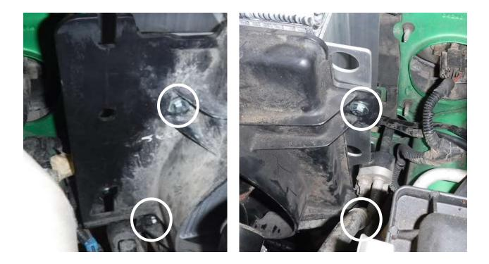
23. Tighten the fan shroud to the radiator using four (4) M6 x 1.0m x 20mm screws, four (4) M6 lock washers, and four (4) M6 fender washers. Tighten to factory specifications.
