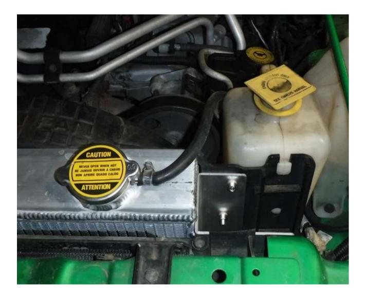
27. Install the coolant reservoir onto the fan shroud.
