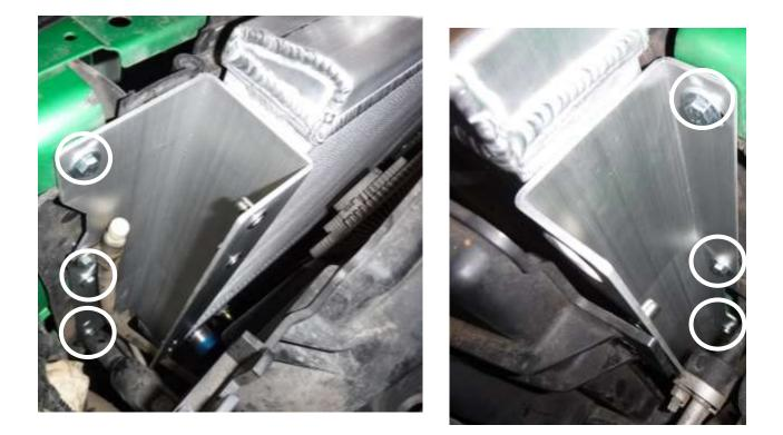
Install the supplied aFe Bladerunner radiator using six (6) supplied M6 x 1.0m x 20mm screws, six (6) supplied M6 lock washers, and six (6) supplied M6 fender washers. Tighten to factory specifications.
