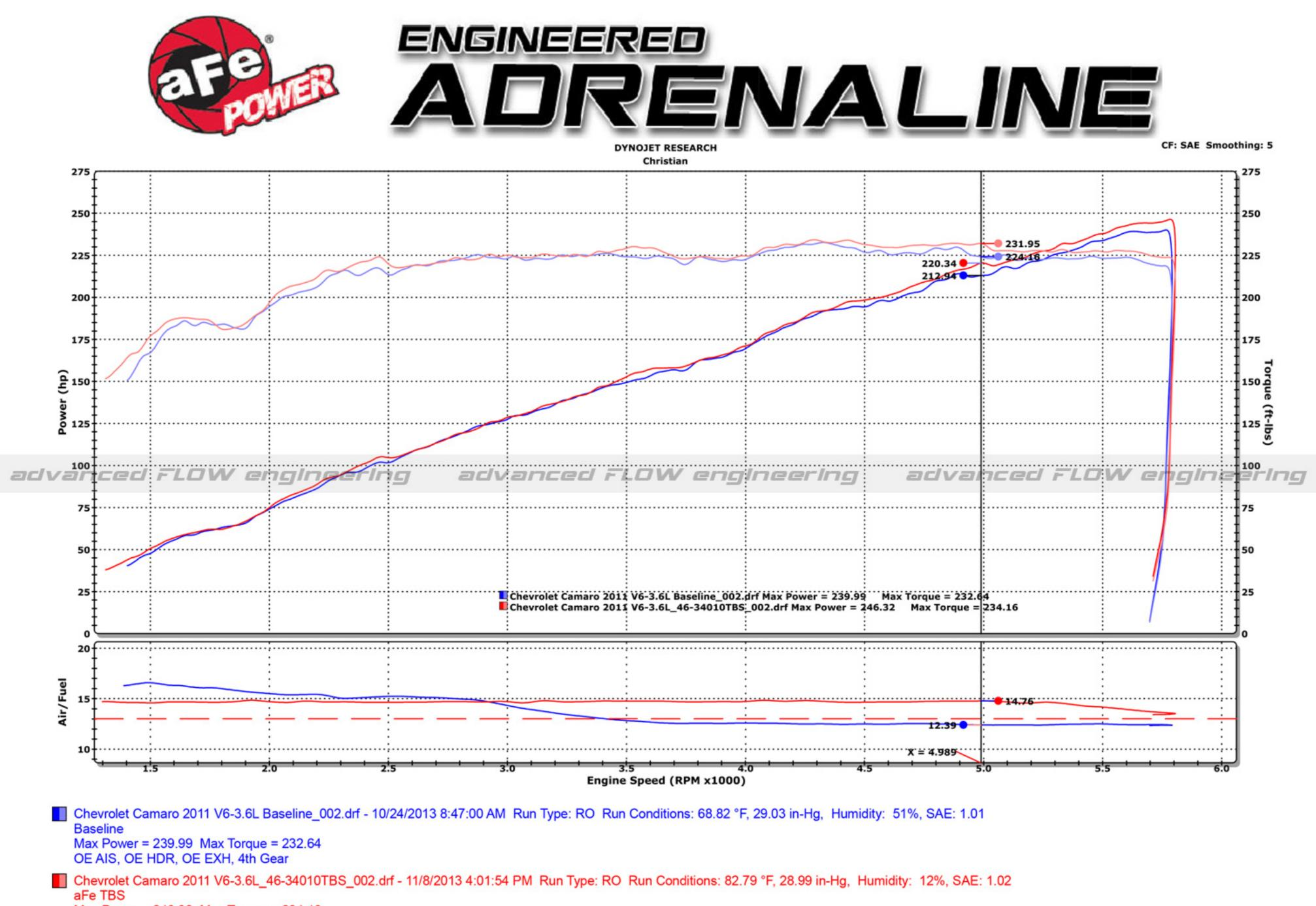
Max Power = 246.32 Max Torque = 234.16 OE AIS, OE HDR, OE EXH, aFe TBS 4th Gear
