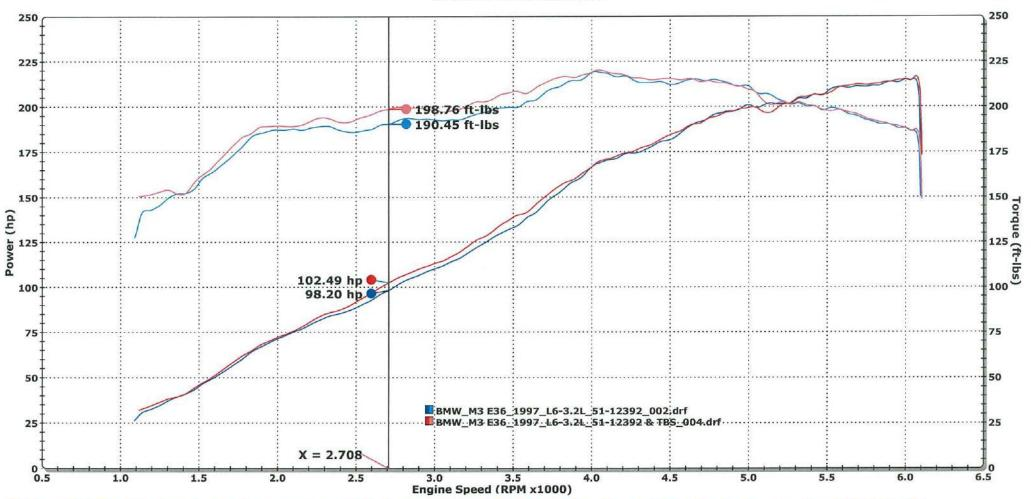
BMW\_M3 E36\_1997\_L6-3.2L\_51-12392\_002.drf - 2/13/2014 1:58:02 PM Run Type: RO Run Conditions: 80.79 °F, 29.03 in-Hg, Humidity: 16%, SAE: 1.02 Max Power = 215.12 Max Torque = 219.35 51-12392 Intake, OE exhaust, No tune 4th gear, 1000-6000RPM
