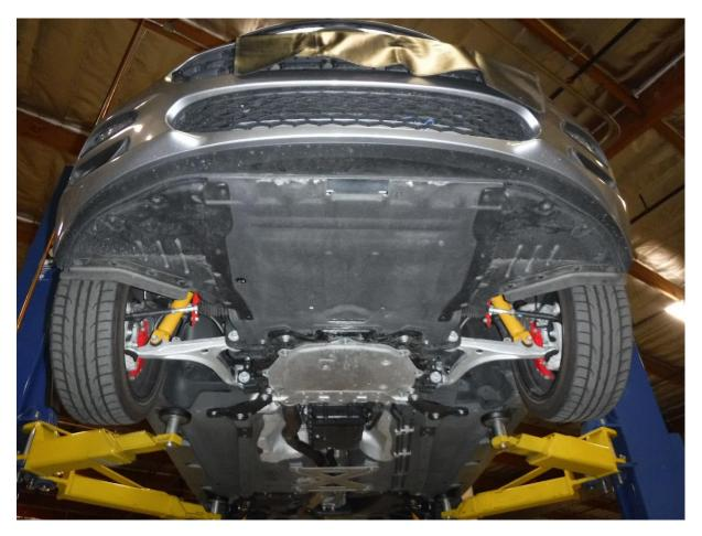
58. Reinstall the skid plate. 59. Reinstall the belly pan.
