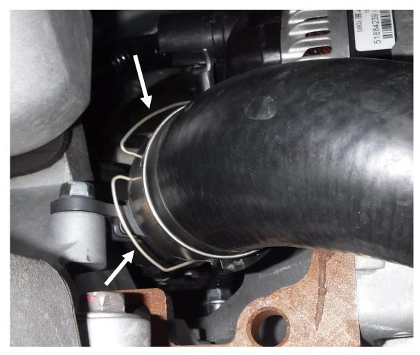
18. To disconnect the quick connect adapter you will need to lift both sides of the retaining clip that secure the intercooler tube to the plastic adapter using two flat head screwdrivers and pull the lower hot side intercooler tube off of the plastic adapter at the same time.
