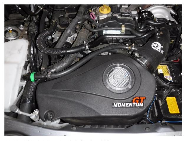
56. Reinstall the intake system back into the vehicle. 57. Reconnect all the vacuum lines.
