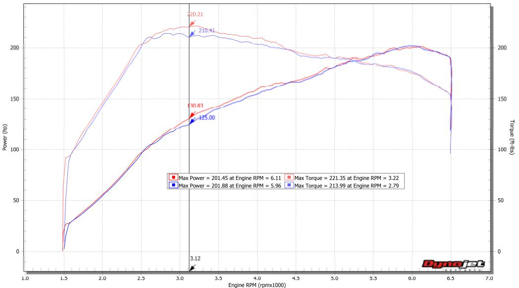
P:\Dyno Runs\Honda\Civic SI\2017\Gamma\Intercooler\Final\Honda\_Civic\_2017\_L4\_1.5l(t)\_IC Tubes\_1.wp8 [ As tested on Dynojet Model 424xLC Linx ][ RPM: OBD2 ] [ AFR Source: Dynoware RT WB ] [ Linx not connected ] [Title: 46-20344 aFe Intercooler Tubes] Notes: Takeda AIS,aFe IC Tubes\_OE IC\_OE Exhaust, 4th Gear, @1.5k RPM, yellow fan & silver fan
