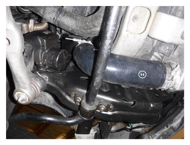
22. Install one (1) of the 3.25" spring-loaded T-Bolt clamps and the supplied 3.38" spring-loaded T-Bolt clamp onto the supplied aFe silicone reducing coupling, 3-1/4" x 3"ID 86 Deg, do not tighten the clamps yet.
