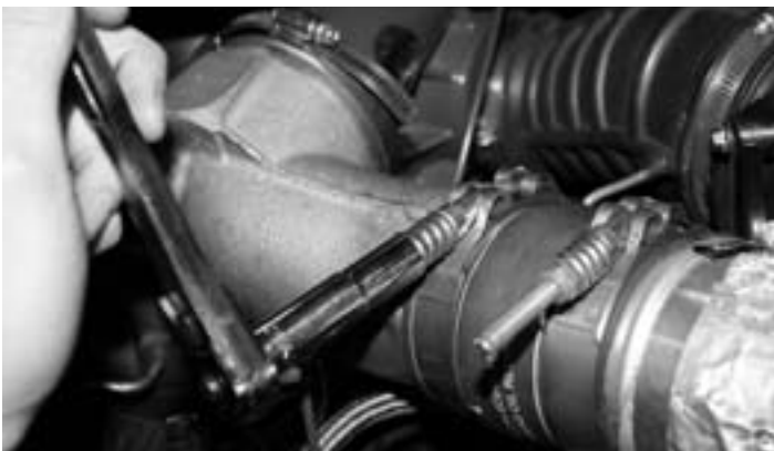
12- Loosen the clamp holding the turbo outlet coupling to the intercooler tube using a 7/16" deep socket.
