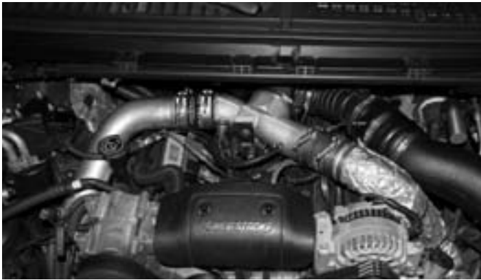
1- View of stock turbo outlet/ intake manifold. Disconnect the negative (-) battery terminals before installation.
