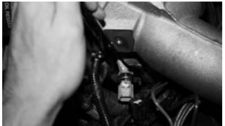
8- Remove the temp sensor from the lower manifold using a 13mm wrench and put aside for later install.
