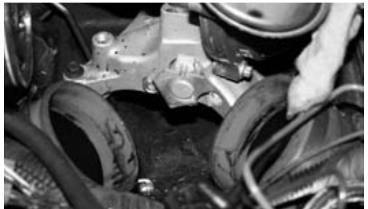
16- Locate the bracket mounting holes that are located directly under these two intake couplings. The holes are on the top of the motor as shown in Step 17.
