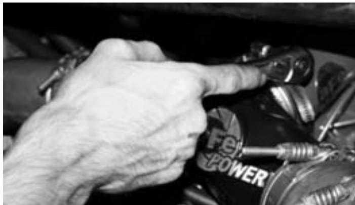
28- Position the turbo outlet manifold onto the turbo evenly and secure with the V-band clamp.
