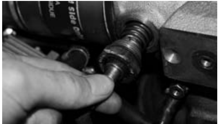
7- Once removed, put the heating element to the side for later install.
