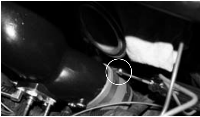
25- Now that you have the manifold in its desired location, tighten both sides of the lower manifold coupling clamps.
