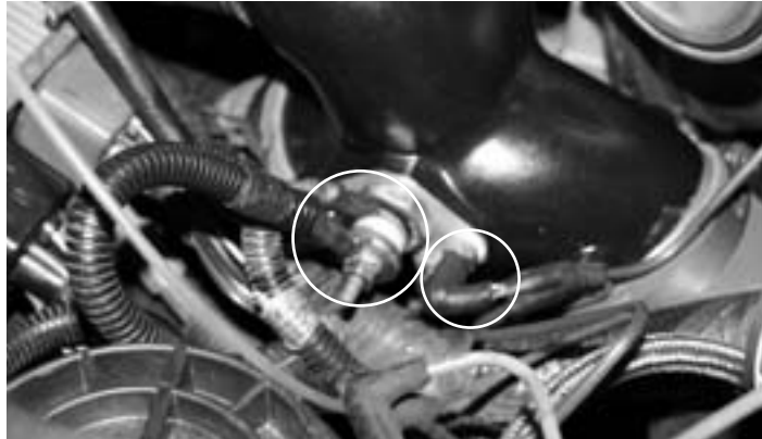
27- Now reinstall the lower manifold wires and hoses that you disconnected in steps #3, #5, and #9.
