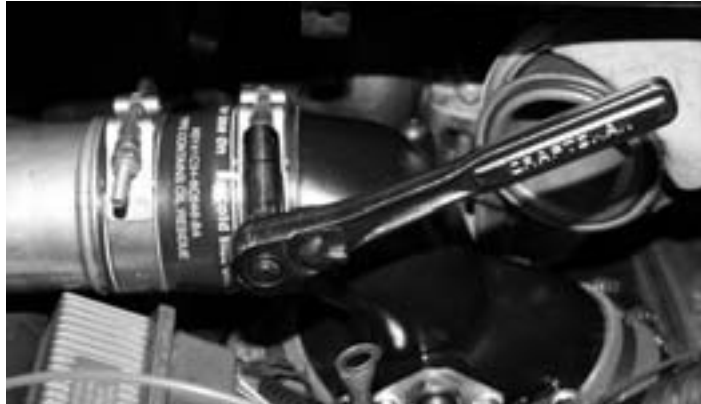
26- Slide the intercooler tube coupling onto the manifold, then tighten clamp. Torque to 9 Ft. Lbs.
