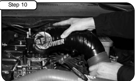
Step 10 Insert aFe manifold into intercooler coupler hose.
