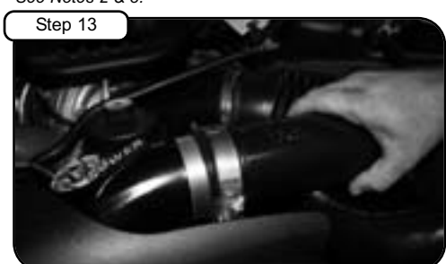
Step 13 Re-attach intercooler tube to manifold.
