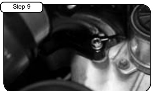
Step 9 With nut and washer provided tighten loosely on manifold screw from step 7.
