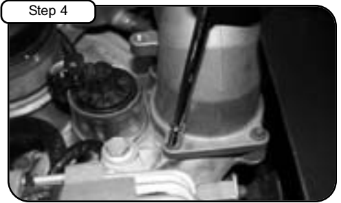
Step 4 With 8mm socket and extension loosen 4 screws holding in manifold.
