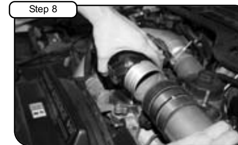
Step 8 Install 1/8" NPT plugs to back of manifold. Tighten using 3/16" allen key. Install new aFe BladeRunner manifold to vehicle. See notes 2 & 3.
