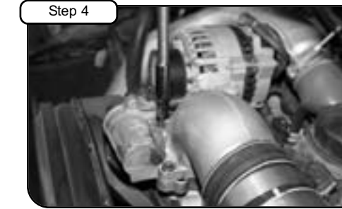
Step 4 With 10mm socket and extension, loosen the 1 screw closest to passenger headlight.
