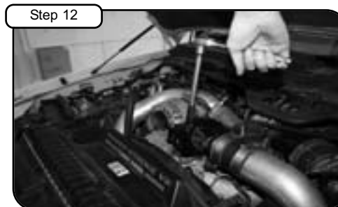
Step 12 Tighten the four mounting screws from Step 11 using 10mm socket. See notes 2 & 5
