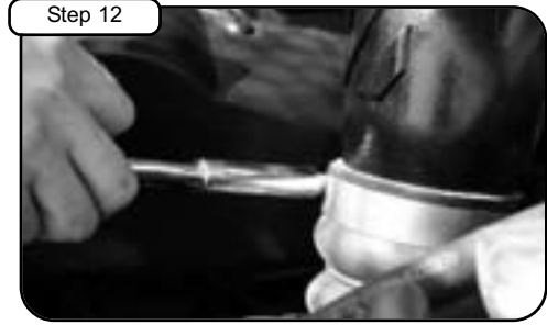
Step 12 Tighten coupler hose clamp with 11mm socket (See notes 2 & 4). Tighten the four mounting screws from Step 11 (See notes 2 & 5).
