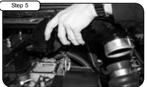
Step 5 Carefully remove stock manifold out of vehicle. ( Place a clean shop rag over air grid heater to prevent anything from entering )
