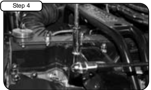
Step 4 With 10mm socket and extension, remove the 4 screws holding the stock manifold.
