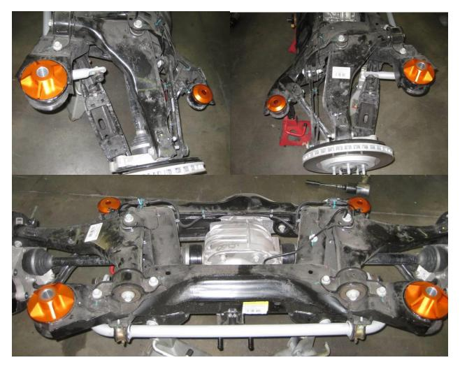
3) Lower the body back on the subframe being careful to align the pins on the body into the mounts.
