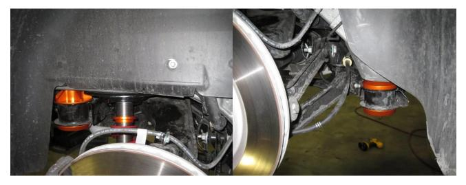
7) Re-install the brake calipers, e-brake lines, driveshaft, lower shock mount and electrical connector
