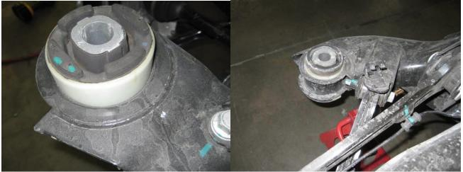
1) With a long, course sawzall blade, cut the rubber and plastic in two places on each bushing all the way to the edge (right up against the subframe). That will release compression on the bushing and allow them to be driven out with a dead blow hammer. They come out easily if they are relieved properly.
