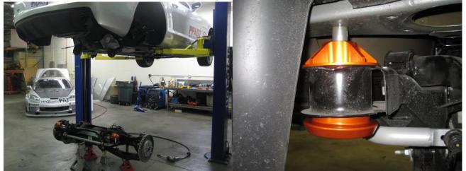
4) Place the lower half of the solid mounts in place and start the bolts by hand.
