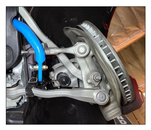
8F Repeat for the passenger side. Clocking and positioning will be a mirror image of the left. Reinstall wheels and torque lug bolts to 103 ft · lbs.
