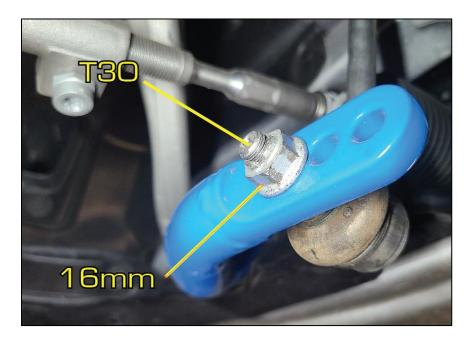
5F Set the aFe Control end link to 15.5" center to center. Make sure to have equal thread engagement for each rod end when adjusting.
