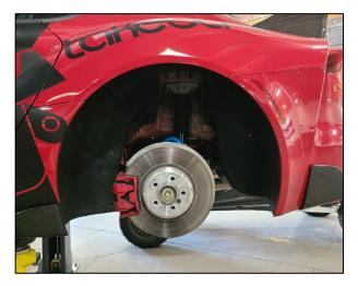
3R Unfasten the left end link from the car using a T30 socket to hold the studs and a 16mm wrench to undo the nuts.
