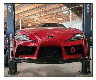
2F Remove the front wheels with a 21mm socket.
