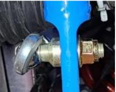
Rotate the entire end link counterclockwise while rotating the bottom rod end clockwise. Back off full clockwise and leaving about 10° of rod end play as a buffer. Tighten the jam nut. Rotate the end link back and forth to make sure there is still about 10° of rod end play.
