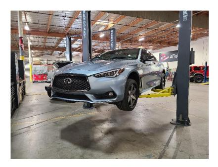
2F Remove the front undertray (16) bolts and (3) pop clips. (10mm socket)
