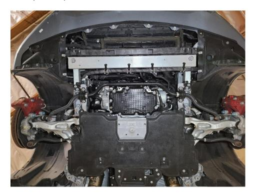
3F Disconnect the end links from the stock sway bar using a 19mm socket for the stud and 17mm wrench for the nut.
