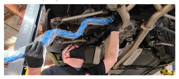
10R Install bushing onto the sway bar. The bushings should be positioned just outside of the centering rings. Slide the aFe Control bushing bracket onto the bushings and mate the sway bar assembly to the subframe. Reuse the factory bolts to secure the brackets to the subframe. Fully tighten this hardware to factory specs.
