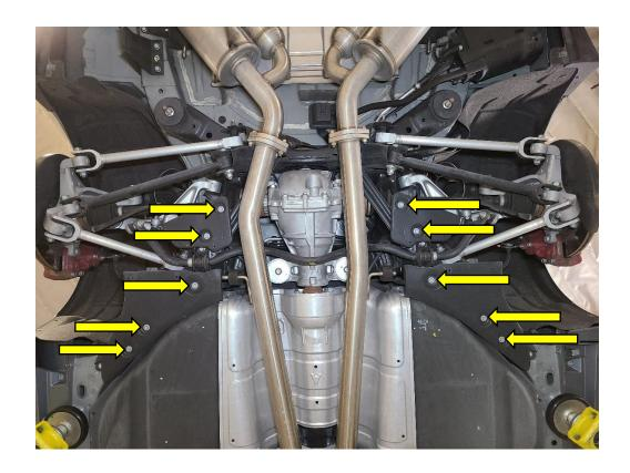
3R In order to have better clearance to install the sway bar remove the exhaust bracket with a 12mm socket to drop the exhaust system low enough for passage.
