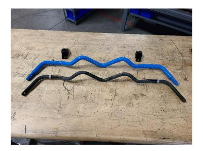
8R Grease the rear bushings with the supplied silicone lube.
