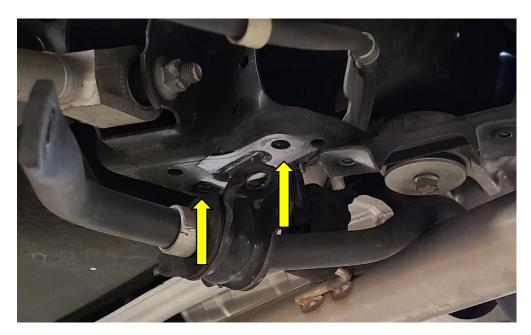
6R Remove the factory sway bar from the vehicle. Note the orientation of the sway bar when removing. (i.e. observe which is the top of the sway bar and how the ends are pointing.)
