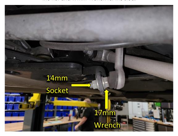
5R Undo the sway bar bushing brackets. (14mm socket)
