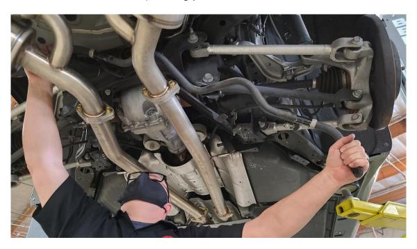
7R Lay out the factory sway bar with the aFe Control sway bar to match the orientation.
