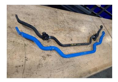
Grease the front bushings with the supplied silicone lube and install bushings onto the sway bar. The bushings should be positioned just outside of the centering rings.
