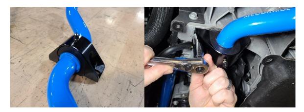
PF Reattach the end links to the sway bar ends reusing the factory nuts. The hole closest to the end is the softest setting. Settings get stiffer as you move away from the ends. (optional: apply thread locking compound to the end link thread)
