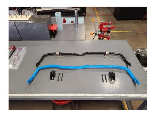
17F Install the front aFe Control sway bar in the same manner as factory removal. We suggest leaving the sway bar in the poly bag when feeding it into the car. This will keep it safe from scratches. (remove the poly bag once bar is in place)
