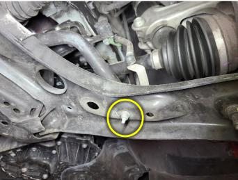
4F Disconnect the end links from the stock sway bar using a (18mm wrench) for the nut and (M6 Triple Square socket) for the stud.
