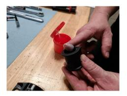
11R Install the bushing onto the sway bar. The bushings should be positioned just outside of the centering rings. Slide the aFe Control bushing bracket onto the bushing. The thin black aluminum spacer goes between the bushing and the subframe. Fully tighten this hardware to 40 ft lbs.
