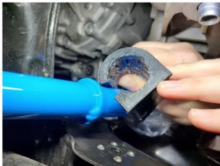
19F Slide the aFe Control bushing bracket onto the bushings with the grease fitting facing out. The thick black aluminum spacer goes between the bushing and the subframe. Use the supplied hardware kit (p/n 00P-0A1713-A) to secure the brackets to the subframe. See diagram below:
