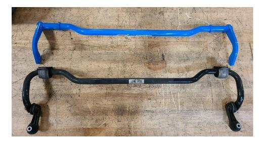
9R Install the rear aFe Control sway bar in the same manner as factory removal. We suggest leaving the sway bar in the poly bag when feeding it into the car. This will keep it safe from scratches. (remove poly bag once bar is in place)
