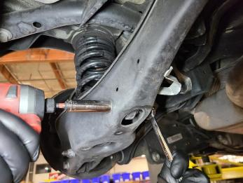
3R Remove the bushing brackets with a (M10 Triple Square).
