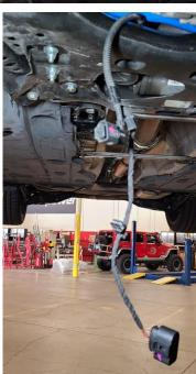
Pry the push-clip to release sensor line from the subframe
