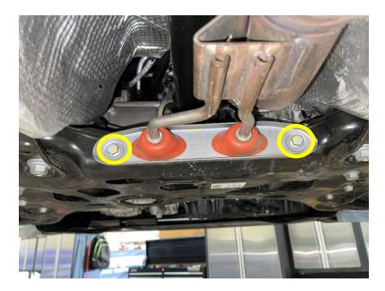
6F Disconnect the engine/trans dog bone mount with a 21mm wrench and socket.
