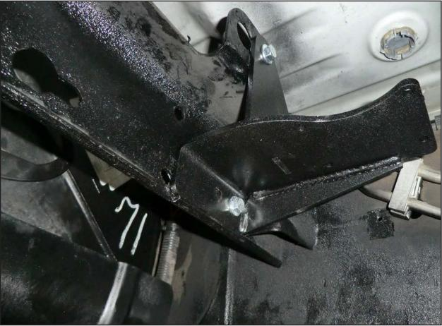
• Mount the carbon steel frame bracket to the frame with the supplied hardware and tighten.
