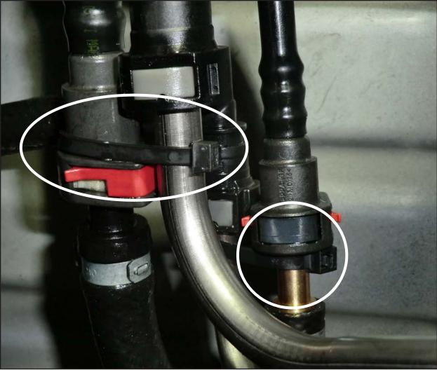
• Using the supplied nylon cable ties, secure the new hoses (as shown above).
