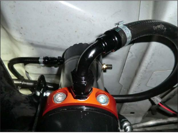
• Install the fuel outlet hose (black 90° -8 AN fitting) onto the male -8 AN fitting on the fuel outlet port of the fuel manifold assembly.
