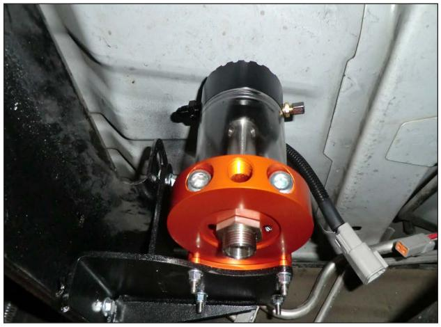
• <u>Mount the supplied fuel manifold assembly</u> to the carbon steel frame bracket using the supplied hardware and tighten.
