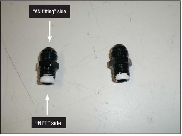
• Apply Teflon tape with PTFE or Teflon paste with PTFE to the 2 x 3/8" NPT to -8 AN fittings.
