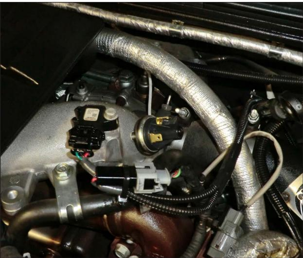
• Install the supplied pressure switch into the intake manifold (1/8" NPT).
