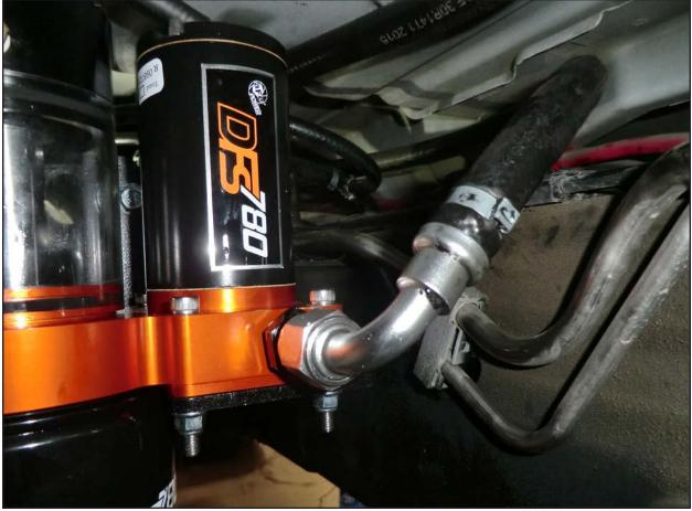
• Install the fuel inlet hose (silver 90° -8 AN fitting) onto the male -8 AN fitting on the fuel inlet port of the fuel manifold assembly.
