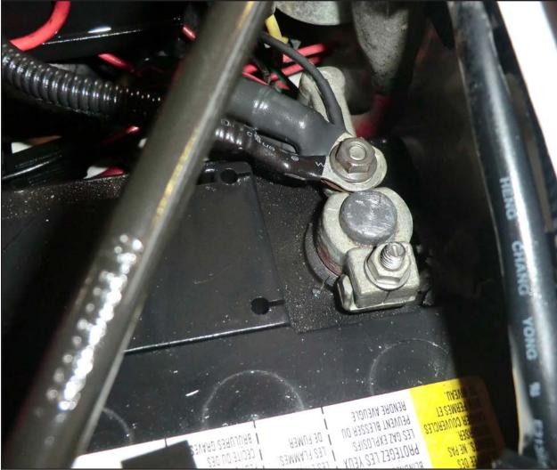
• Connect the black wire ring terminal on the power harness to the negative side of the battery.
