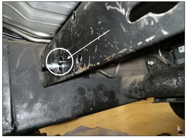
**NOTE:** Make sure the pin in the bracket goes through the bracket on the frame (shown above).
