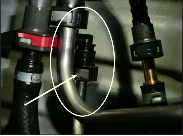
• Install the 90° female quick disconnect fitting on the fuel return hose onto the male side of the stock fuel return line.
