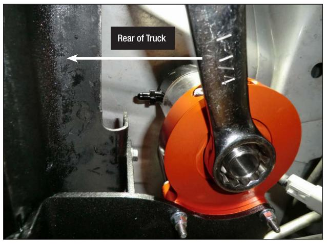
• Turn the sight glass to the desired angle and using a 1-1/4" wrench, tighten the center nut under the fuel manifold assembly.
