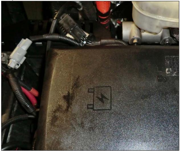
$\bullet$  Secure the relay harness using a supplied nylon cable tie.
