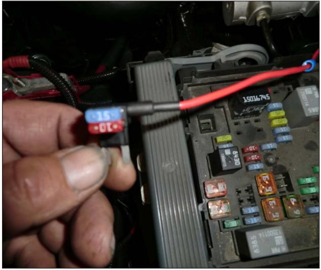
• Install the fuse removed on page 28 into the open location on the add a harness fuse adapter (not in line with the wire).
