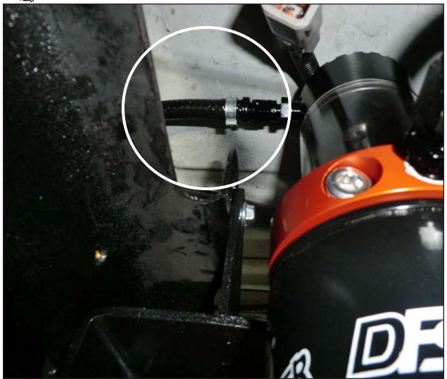
• Install the fuel return hose (-4 AN fitting) onto male -4 AN fitting on the top of the sight glass cover.
