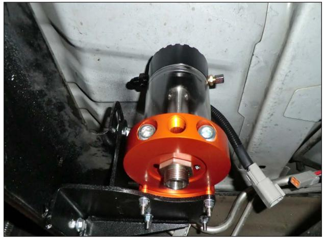
• Mount the supplied fuel manifold assembly to the carbon steel frame bracket using the supplied hardware and tighten.
