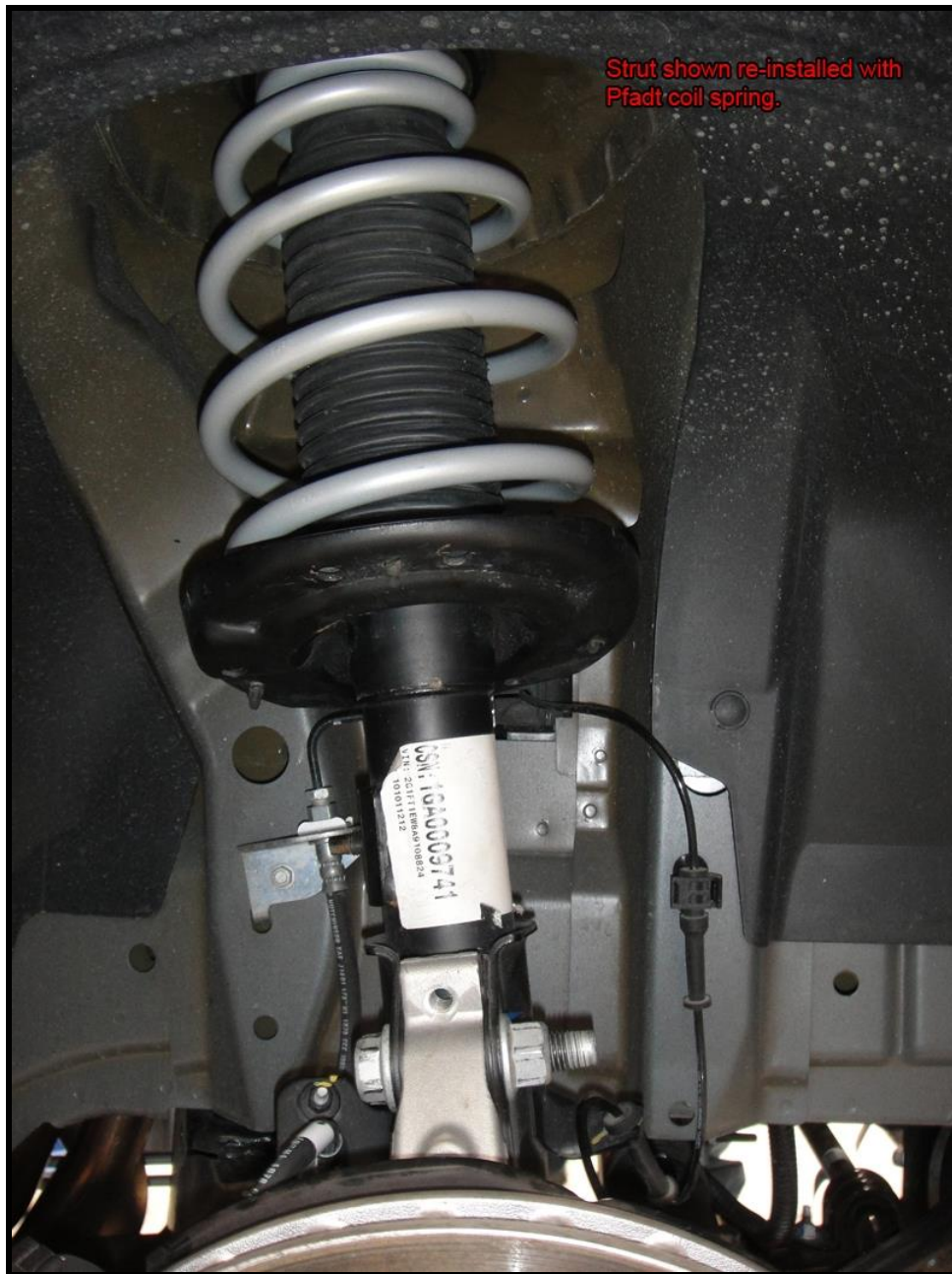
Figure 8 - Front Strut with Pfadt Drop Spring
