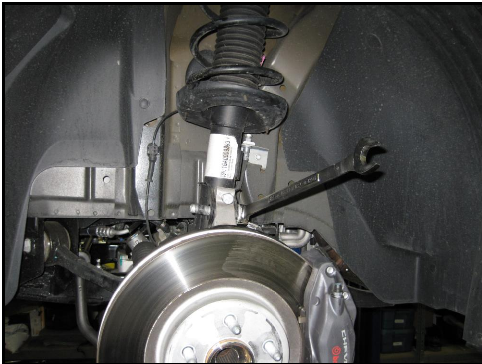
Figure 4 - Removing Spindle to Strut Bolts
