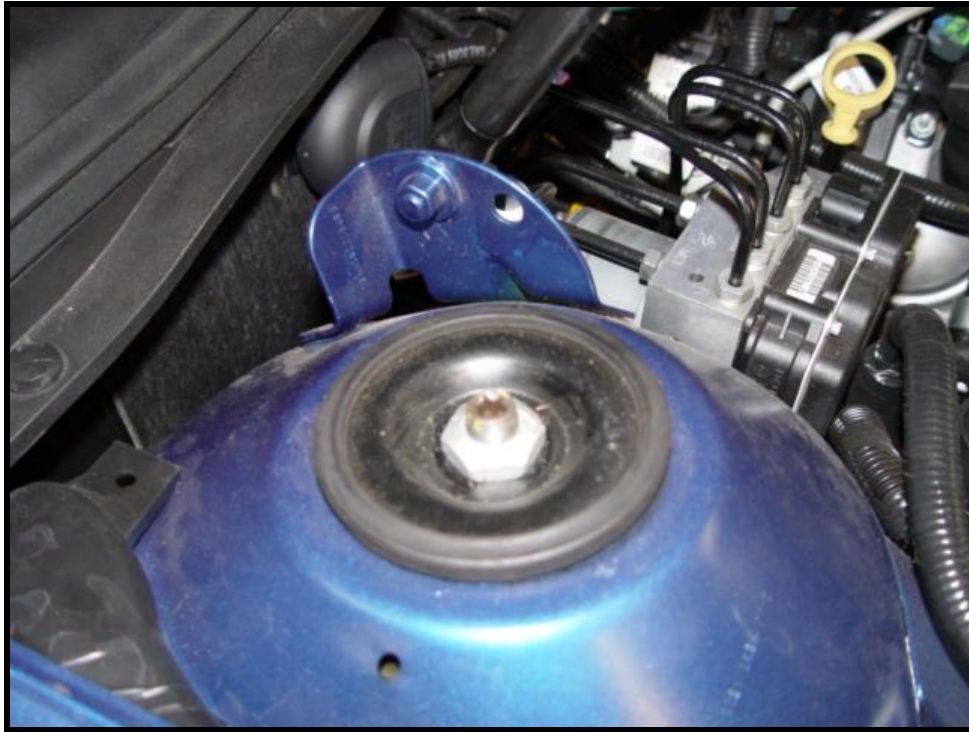
Figure 2 - Upper Nut and Strut Retaining Plate
