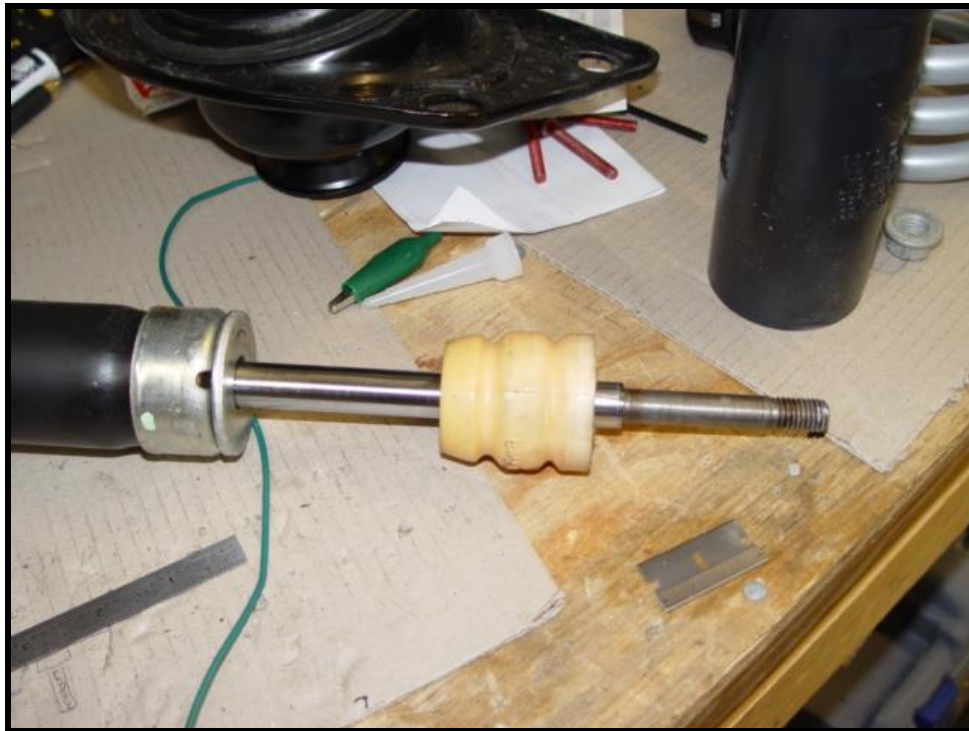
Figure 14 - Strut with un-cut Bump Stop
