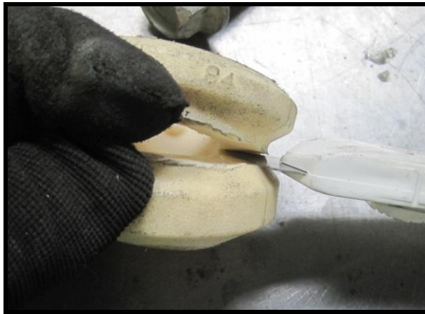
Figure 7- Trimming Front Bump Stop
