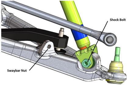
Using the Sharpie marker, mark the rotation of each of the camber adjustment eccentrics that mount the lower control arms to the subframe. These marks will be used to get a baseline adjustment upon re-assembly.
