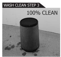
Allow the filter to dry completely (our synthetic media dries quickly and should dry within a few hours in normal conditions). Reinstall the filter in your vehicle. Do not apply oil to the filter.
