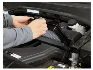
3. Slide aFe air filter into the airbox.
