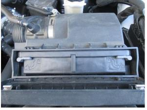
1. Open the air filter access panel. Rotate the locking tabs to unlock position; and pull out the stock filter.
