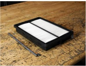
2. Pop out the rods from stock air filter, you will need these for the installation of the aFe air filter. Please note, the rods are left and right specific.
