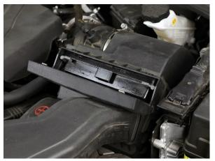
5. Rotate the tabs to the locked position as shown on air filter. Close the air filter access panel.
