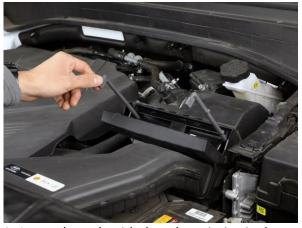
4. Insert the rods with the tabs pointing in the unlock position under the outermost edge of the filter.
