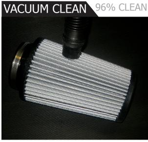
You can vacuum your Pro Dry S filter and return it to 96% of its original airflow. Remove the filter from the intake kit and vacuum away the dirt using a shop vacuum or regular house vacuum. Reinstall the filter in your vehicle. Do not apply oil to the filter.
