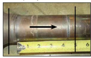
Install the aFe direct fit catalytic converter replacement using the OE V- band clamp, but do not tighten. Slide the adapter pipe over aFe Step 7:
