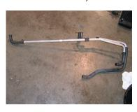
14. Remove the factory bracket assembly from the factory heat exchanger by removing the (4) bolts from the bottom bracket.
