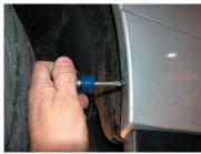
Remove the 2 bolts securing the power steering cooler and lower the cooler out of the way.
