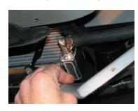
22. Reposition and attach the RH shield next to the heat exchanger hose connections.
