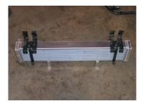
18. Install the AFCO Heat Exchanger assembly into the vehicle just like the factory unit was installed. Install the (4) bolts from the grill opening and tighten.
