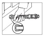
Step 2. Push the sleeve over the end of the tube and under the wire braid by hand. Complete positioning of the sleeve by pushing the hose end against a flat surface. Visually inspect to see that the tube butts against the inside shoulder of the sleeve. Set the sleeve barbs into the Teflon\* tube by pushing a round nose tapered punch into the end of the sleeve and tube.
