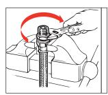
Step 4. Wrench tighten hex until clearance with socket hex is at .031 inches. Your thumbnail is a convenient measuring device. Tighten further to align corners of nipple and socket hexes. CLEAN, PROOFTESTTOTWICE
