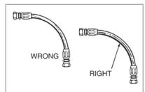
If a hose is installed with a twist in it, operating pressures tend to force it straight. This can loosen the fitting nut. Twisting can cause reinforcement separation, and the hose could burst at the point of strain.
