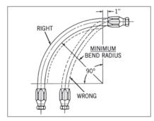
At bends, provide sufficient hose so that it does not have a bend radius less than its recommended minimum bend radius. Too tight a bend may kink the hose and restrict or stop the fluid flow. In many cases, the proper use of adapters and hose fittings can eliminate tight bends or kinks.
