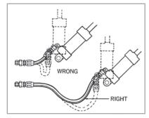
In applications where there is considerable vibration or flexing, allow additional hose length. Metal hose fittings, of course, are not flexible, and proper installation protects metal parts from undue stress and avoids kinks in the hose.
