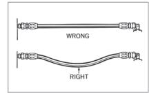
Under pressure, a hose may change in length. Always provide some slack in the hose to allow for this shortening or elongation. (However, excessive slack in hose lines may cause poor appearance.)
