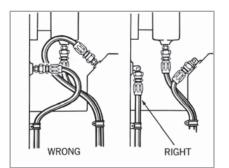
When 90° adapters were used, this assembly became neater-looking and easier to inspect and maintain. It uses less hose, too!
