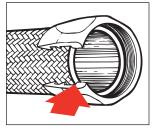
Step 2. Insert hose in socket with twisting, pushing motion until hose is in line with back of socket threads.
