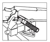
Step 1. Cut hose square to length with fine-tooth hack saw or cut-off wheel. To minimize wire braid flare out, wrap hose with masking tape and cut through tape. Remove tape before next step.
