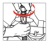
Step 5. Carefully insert nipple and engage nipple and socket threads while holding hose in position with other hand. Make sure hose does not push out of socket by observing mark made in Step 3.
