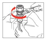
Step 6. Complete assembly using wrench while continuing to hold hose in position. Maximum allowable gap is .031 inches. Your thumbnail is a convenient measuring device.
