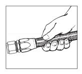
Step 7. Important—Check hose for pushout by observing hose position mark. Pushout should not be evident. CLEAN, PROOF TEST TO TWICE OPERATING PRESSURE AND INSPECT ALL ASSEMBLIES.
