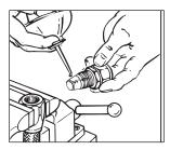
Step 4. Lubricate inside of hose and nipple threads liberally using S.A.E. 30 lubricating oil or Aeroquip FBM3553 Hose Assembly
