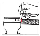
Step 3. Important—Mark position around hose at rear of socket with a grease pencil, paint or tape.
