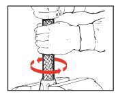
Step 2. Put socket in vise. Screw hose counterclockwise into socket until it bottoms. When assembling long lengths of hose, it may be preferred to put hose in vise just tight enough to prevent from turning, and screw socket onto the hose counterclockwise until it bottoms. Back off 1/4 turn.
