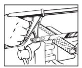
**Step 1**. Cut hose square with fine-tooth hacksaw or cut-off wheel.
