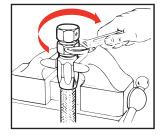
Step 4. Male Ends: Screw nipple clockwise into socket and hose. Leave a 1/32∀ clearance between nipple hex and socket
