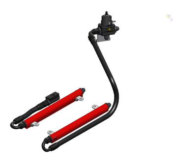
27. Assemble a hose with a straight AN-08 hose end on one end with a 180 degree hose end on the other. Attach this hose to the front of the passenger side rail using the 180 degree end. Place the pressure sensor re-locator on the other end as pictured.
