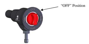
4. When a fuel sample is needed, rotate the red locking knob to the "ON" or unlocked position and press the knob until the desired sample is acquired. After the desired sample has been taken return the red locking knob to the "OFF" or locked position.
