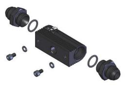
22. Thread the o-ring side of the remaining four p/n 15607 port fittings into each end of each fuel rail.
