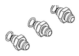
27. Thread the port (o-ring) side of the 15606 port fittings into each of the three ORB-06 ports on the regulator.
