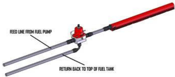
Fuel Rail with single inlet (Figure 1-1)
