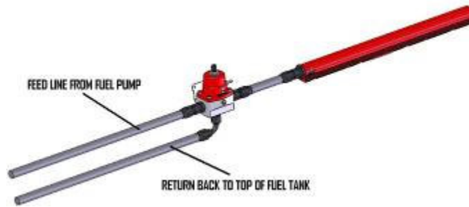
Fuel Rail with single inlet (Figure 1-1)
