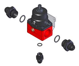
25. Install one ORB-08 o-ring on the port (cut-off) side of each of the four P/N 15607 ORB-08/AN-08 port fittings.
