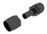
D. Using a grease pencil, marker or tape, mark the location of the hose in relation to the hose socket which you just installed.
