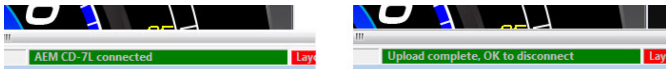
Figure 6 - Status bar in DashDesign software. Do NOT disconnect USB cable until OK to disconnect message is shown.
