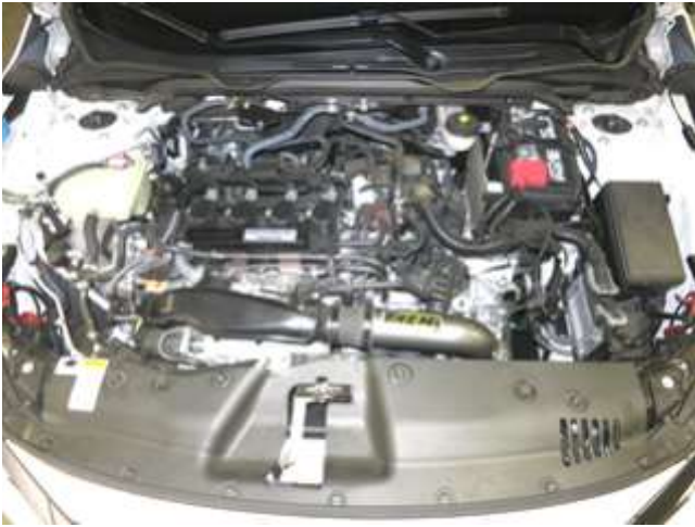
STOCK CHARGE PIPE INSTALLED
