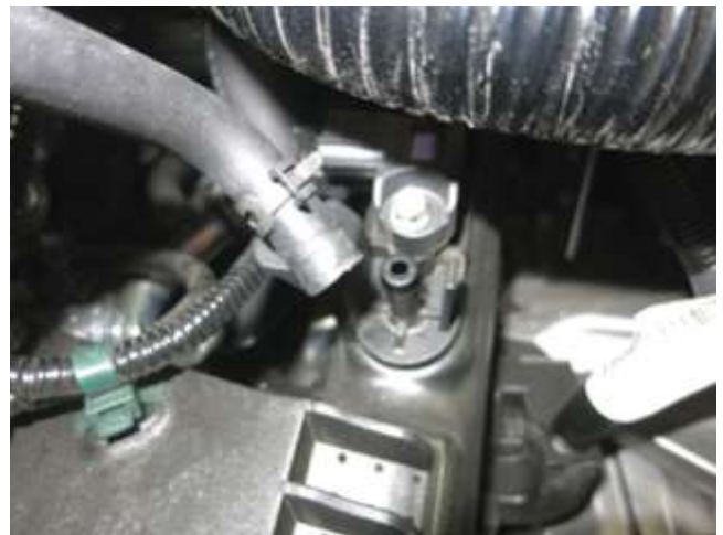
d. Use pliers to pinch the spring clamp and pull the vacuum hose from the stock charge pipe nipple.
