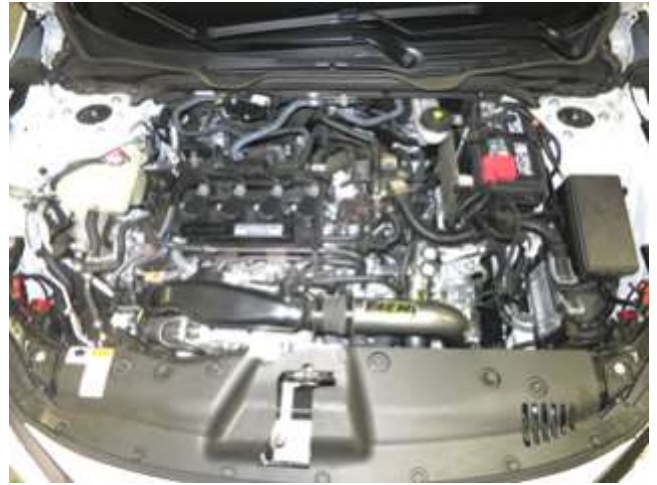
AEM CHARGE PIPE INSTALLED
