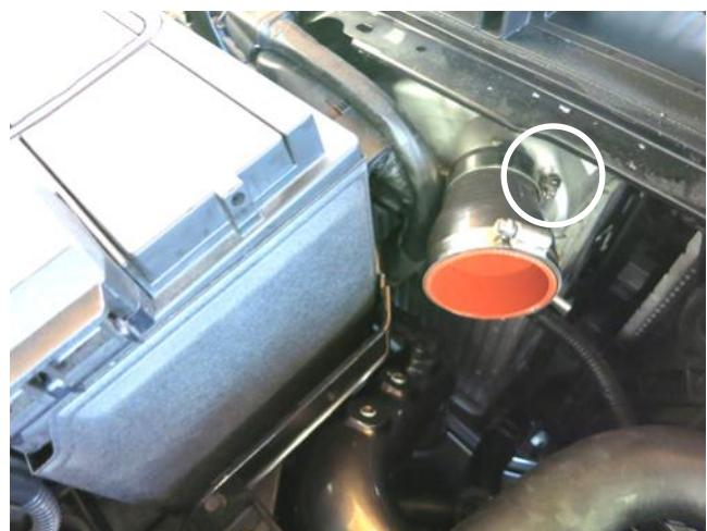
h. Install the provided coupler and hose clamps onto the intercooler. Tighten the hose clamp circled at this time to 30 in-lbs.
