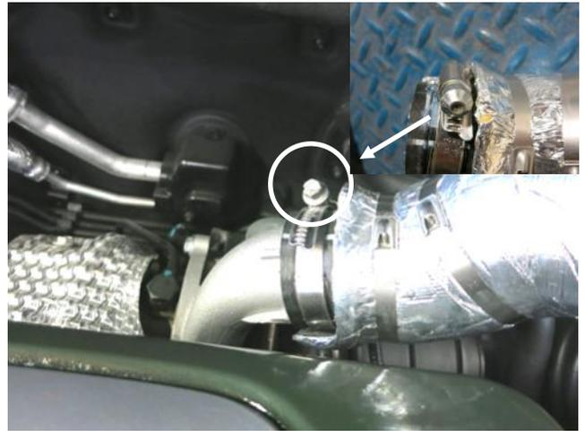
f. Loosen the hose clamp at the turbo compressor. Note: A hose clamp cap that covers the slot may be present. You can pry it off with a screwdriver or pliers.
