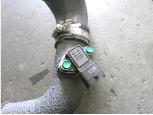
n. Remove the two M6 bolts securing the pressure sensor to the lower intercooler pipe. These bolts will be reused in step 3a.
