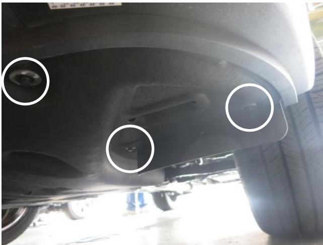
k. Remove the 17 bolts that secure the splash shield to the vehicle. Note: The small oil access cover does not need to be removed from the shield and not all of the bolts are pictured above.
