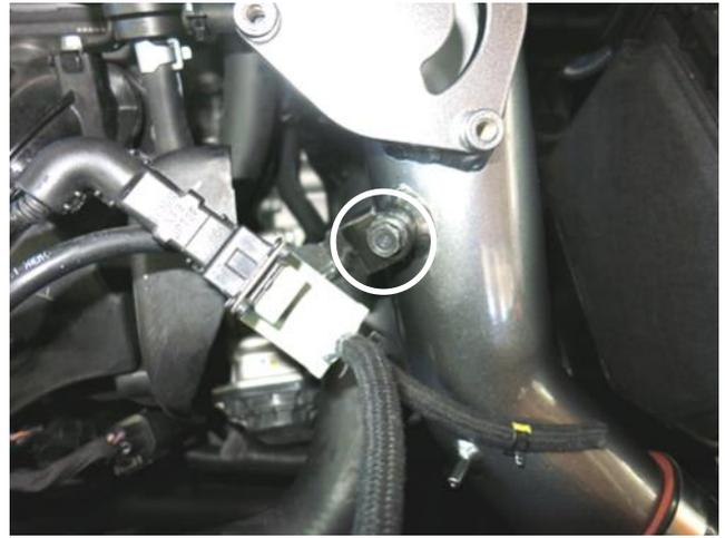
l. Using the bolt removed in step 2c to secure the electrical connector to the AEM pipe.
