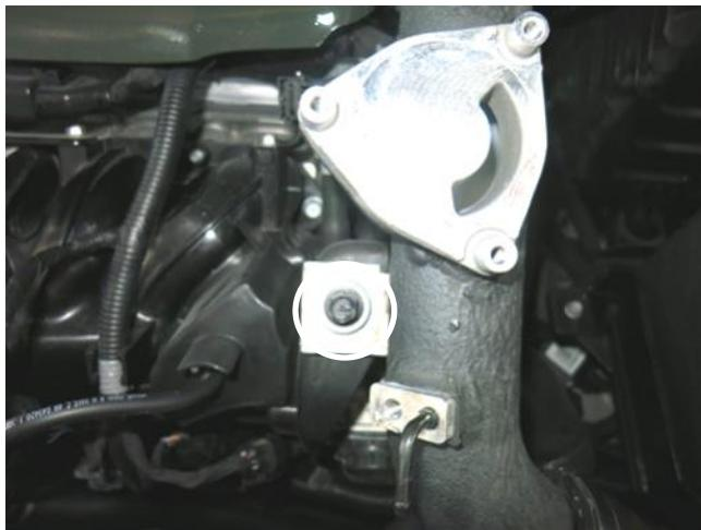
e. Remove the bolt that secures the intercooler pipe to the engine. This bolt will not be reused.
