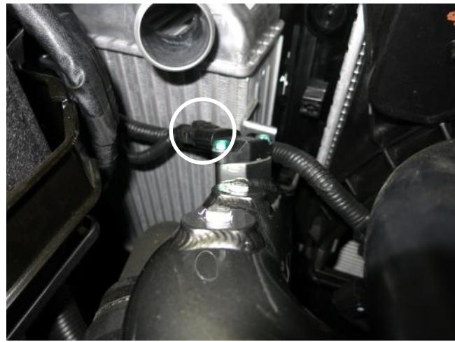
f. Connect the pressure sensor electrical connecter to the pressure sensor.
