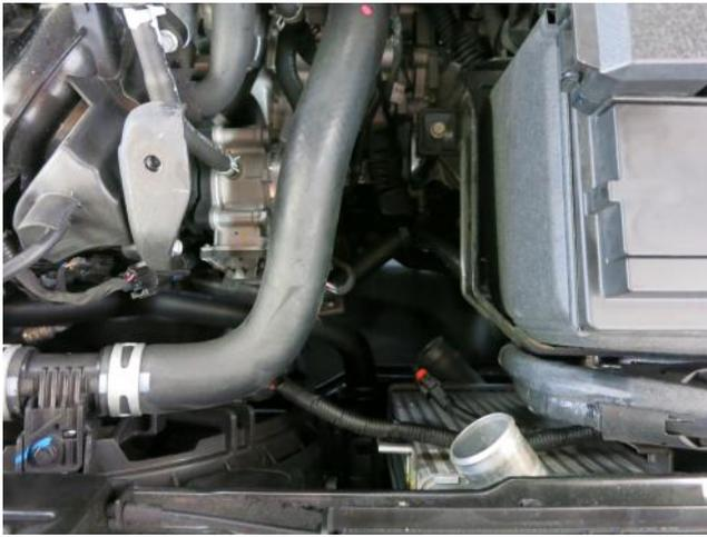
m. Remove the lower intercooler pipe from the vehicle, disconnecting it from the lower intercooler first, then from the throttle body, finally taking out from the top.
