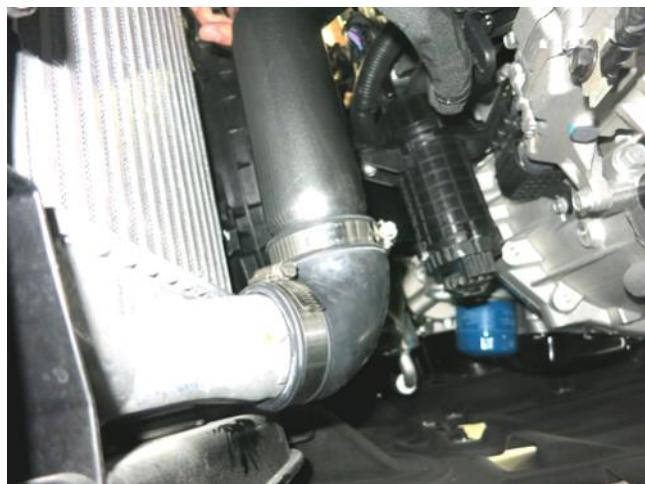
c. Install the AEM intercooler pipe into the coupler. Tighten hose clamp once upper part of tube is aligned to 30 in-lbs.
