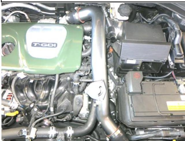
i. Install the AEM upper intercooler pipe into the previously installed coupler on the intercooler first, then into the coupler. Note: Using warm soapy water may help installation and alignment.
