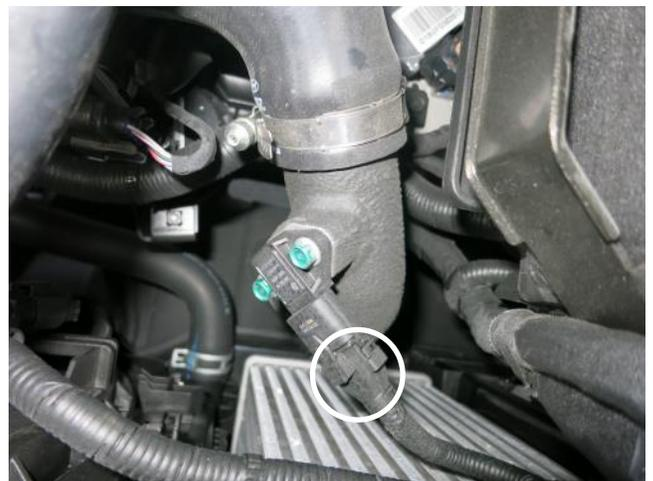
j. Remove the electrical connector from the pressure sensor on the lower intercooler pipe.
