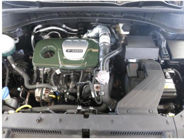
STOCK CHARGE PIPES INSTALLED
