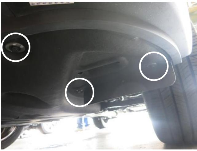
q. Reinstall the splash shield and the 17 bolts to the vehicle. Note: Not all of the bolts are pictured above.
