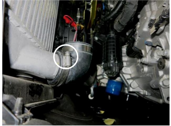
b. Install the 90° coupler with the provided hose clamps onto the lower intercooler outlet. Note: Warm soapy water will help with installation.
