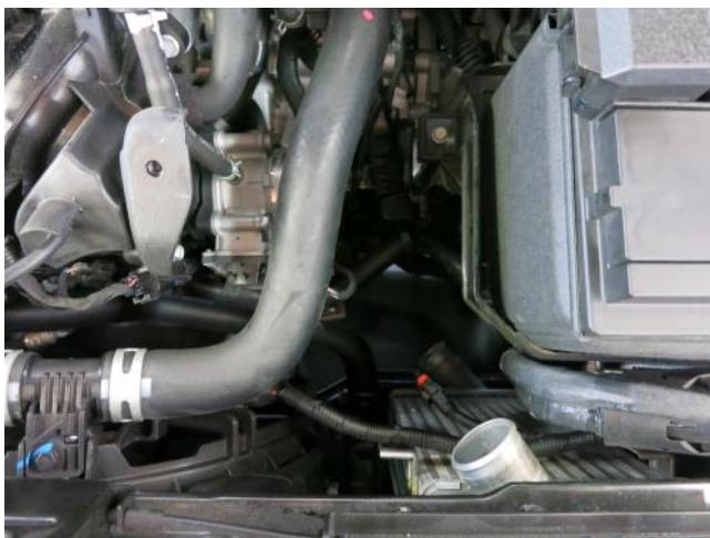
m. Remove the lower intercooler pipe from the vehicle, disconnecting it from the lower intercooler first, then from the throttle body, finally taking out from the top.
