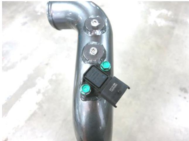
a. Install the 2 NPT plugs into the AEM intercooler pipe with Teflon tape or pipe sealant. Then, install the pressure sensor with M6 bolts removed in step 2n.
