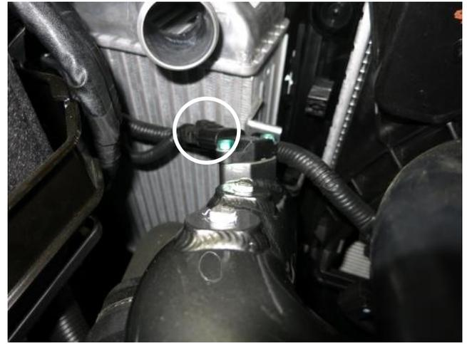
f. Connect the pressure sensor electrical connector to the pressure sensor.
