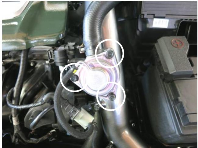
n. Reinstall the BOV onto the AEM intercooler pipe and tighten with the bolts that were removed in step 2d.
