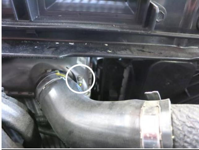
g. Loosen the hose clamp at the intercooler. Note: A hose clamp cap that covers the slot may be present. You can pry it off with a screwdriver or pliers.
