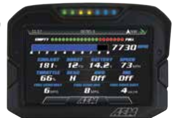
A Vehicle Diagnostics page displays all channels for monitoring/troubleshooting.
