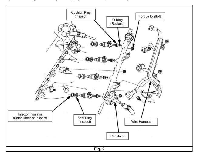
j) Inspect all seals, o-rings, and washers. If any of these components look at all worn or damaged, then replace with genuine Honda parts.
