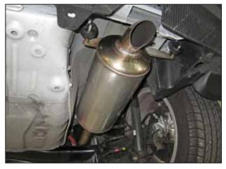
c. Install the rear section of the AEM $^{\circ}$  exhaust (83035) as shown, by engaging the two rubber mounts at the muffler.
