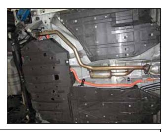
g. Install the AEM $^{\odot}$  mid pipe (83034) as shown by engaging the two rubber mounts.
