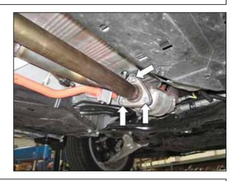
i. Secure the mid pipe to the OEM catalytic converter with the three supplied M10 nuts (RHNA-M10X125).
