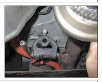
d. Disengage the rear most rubber mount on the mid pipe by sliding it off of the mount on the vehicle's side.
