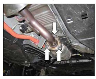
a. Remove the 3 nuts securing the OEM mid pipe to the catalytic converter.
