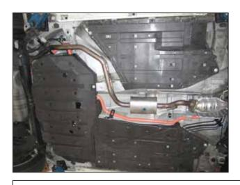
e. Disengage the remaining two rubber mounts and remove the mid pipe from the vehicle.
