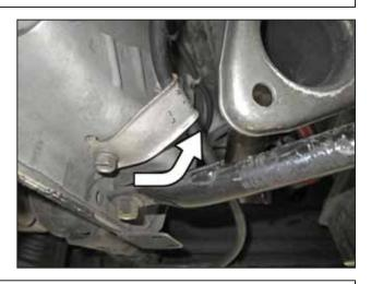
e. Bend the emergency brake bracket up out of the way as shown.
