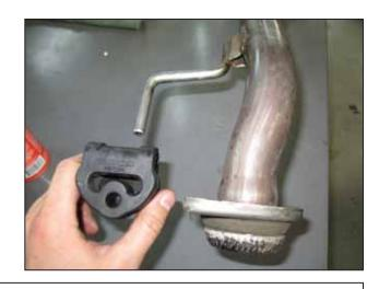
f. Remove the rear most rubber mount from the mid pipe as shown. Silicone spray will help with the removal.
