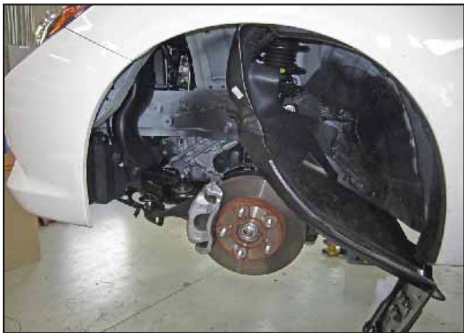
y. Move the fender liner aside to gain access to the fenderwell.
