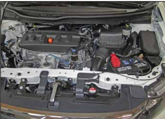
Stock air box system installed.
