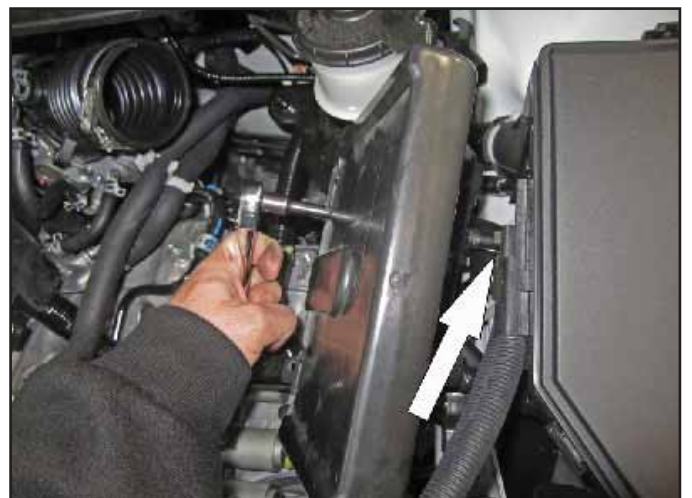
n. Move the ECU to gain access to the remaining 10mm bracket bolt. Remove bolt.
