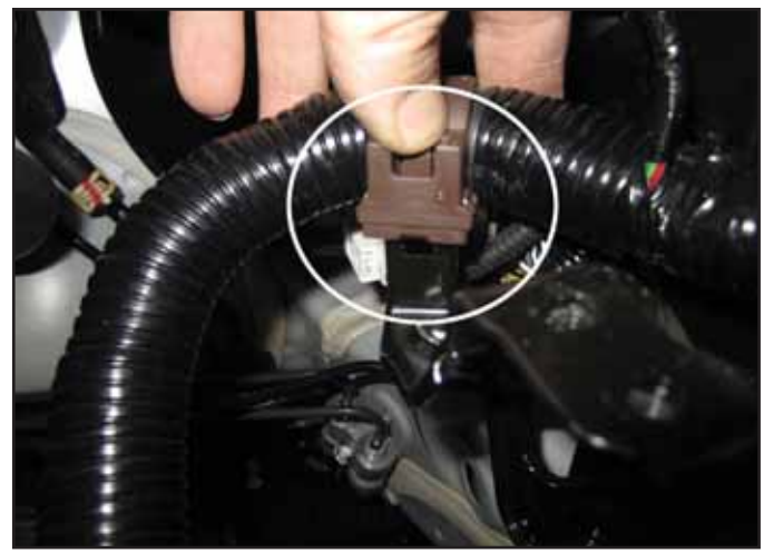
p. Release the wire harness clip from the bracket.
