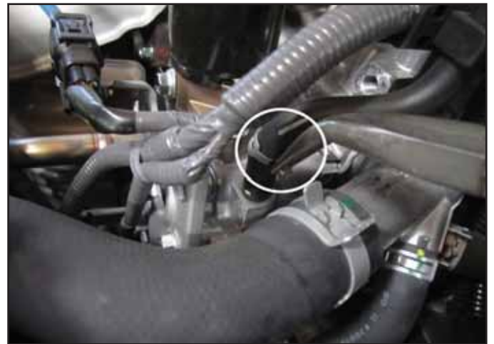
ad. Release the clip on the thermostat housing hose and move upward. (The car must be cool before proceeding with this step).
