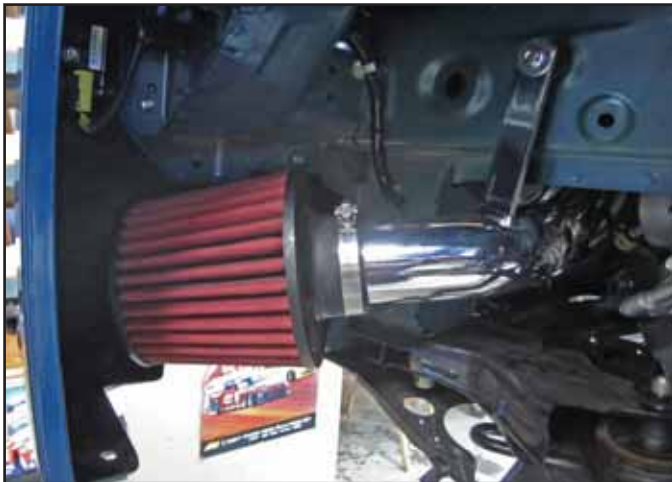
n. Install the AEM® Air Filter onto the lower intake tube and tighten the #44 hose clamp.
