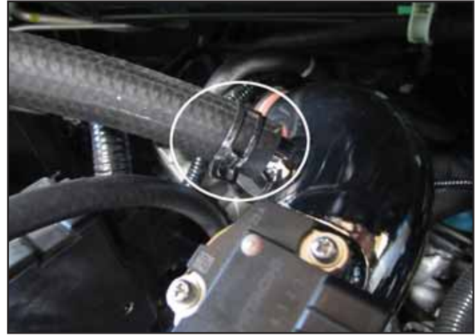
s. Install the PCV hose with the OEM clip onto the intake tube.
