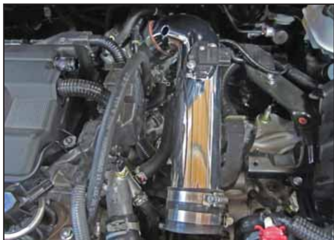
j. Install the intake tube into the throttle body, but do not tighten the hose clamp.
