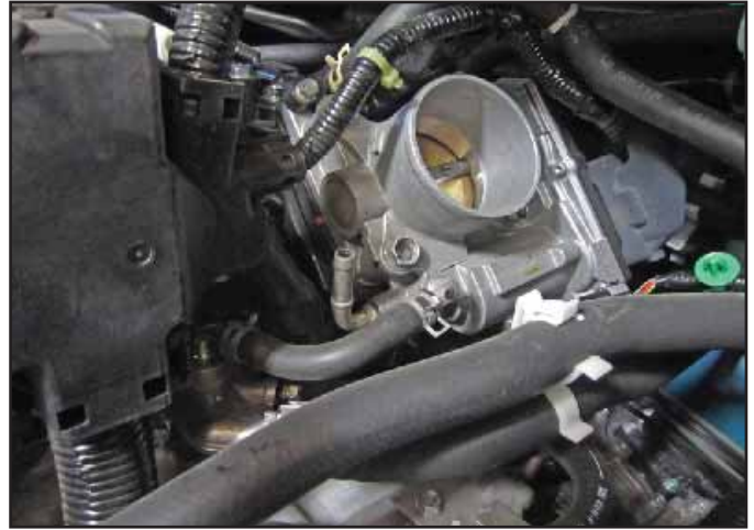
ag. Remove the coolant hose from the throttle body.
