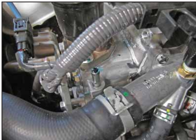
ae. Remove the coolant hose from the thermostat housing. (Have some rags nearby to absorb any spilled coolant).
