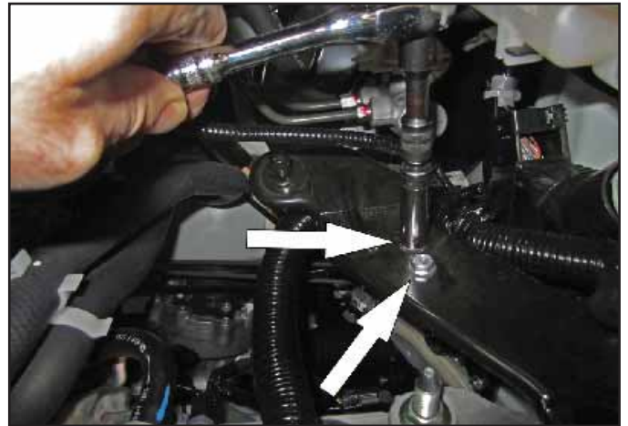
j. Remove the back two 10mm bolts securing the air box bracket.
