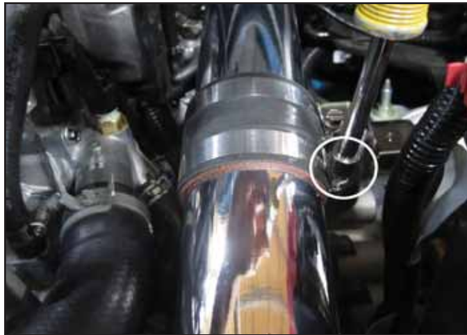
p. Tighten the hose clamp on the lower intake tube.
