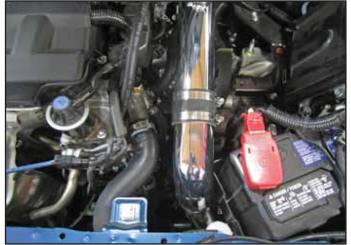
m. Align the upper and lower intake tubes, but do not tighten the hose clamp.
