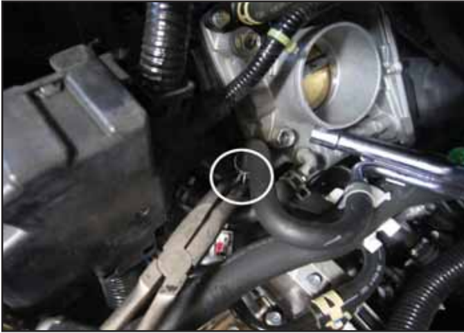
af. Release the clip on the throttle body hose and move upward.
