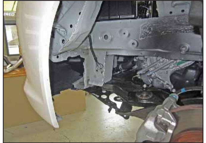
ab. Remove the resonator tube.
