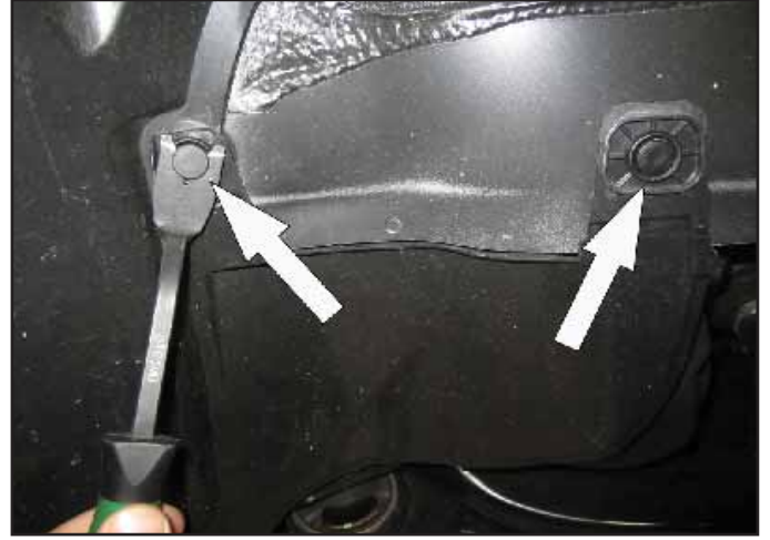
v. Remove the two plastic clips securing the side splash shield.
