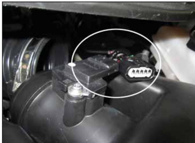
g. Disconnect the mass air flow sensor.
