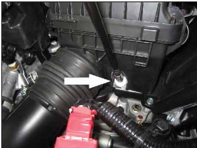
a. Remove the front 10mm bolt securing the factory air box.
