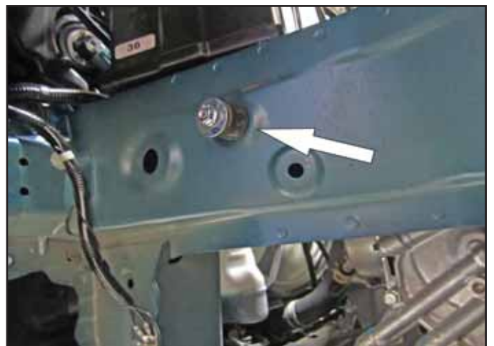
k. Install the rubber mount with 6mm washer and nut.
