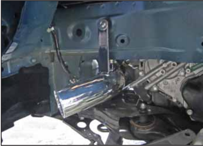
l. Install the lower intake tube.
