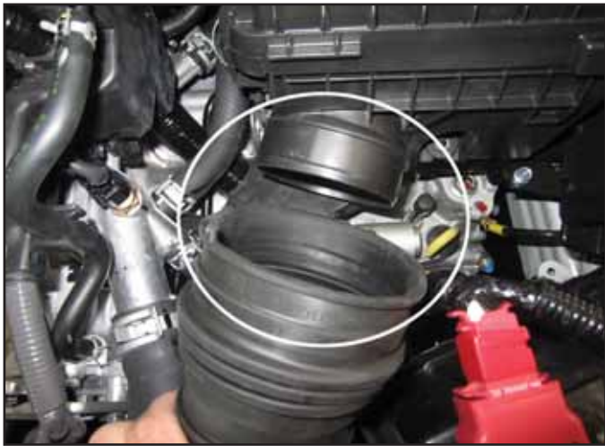
c. Disconnect the air duct from the front of the factory air box.
