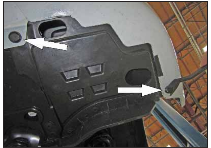
x. Remove the two plastic clips securing the fender liner.
