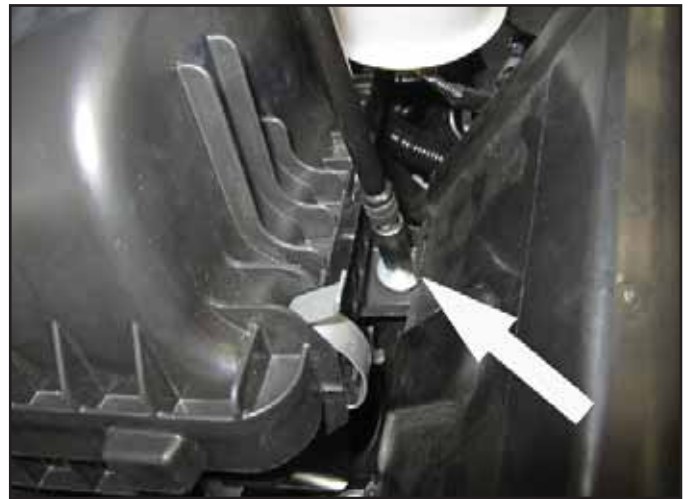
b. Remove the right 10mm bolt securing the factory air box.
