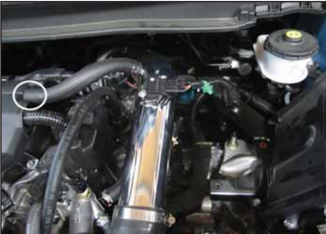
t. Install the PCV hose onto the valve cover.
