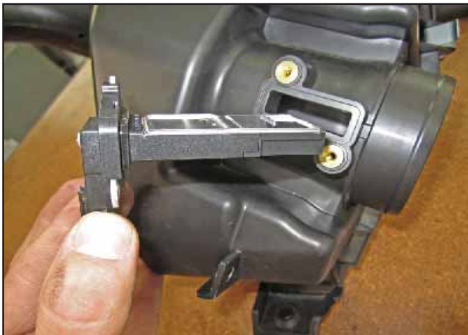
ac. Remove the mass air sensor from the air box.
