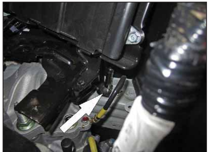
l. Remove the lower 10mm bracket bolt.
