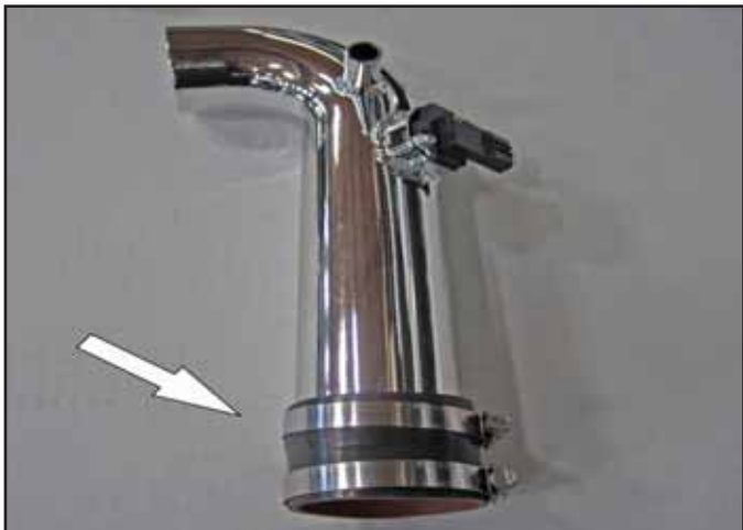
h. Install the coupler and two #40 hose clamps onto the upper intake tube.
