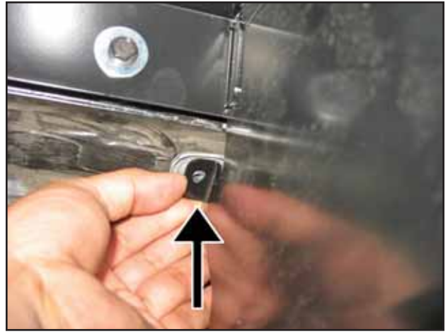
k. Insert the supplied spacer between the hole on the lower part of the heat shield and the threaded hole exposed in step 2q.
