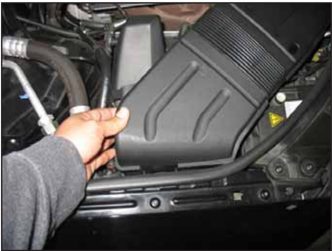
c. Carefully lift the back side of the fresh air duct away from the air box.
