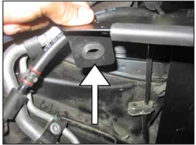
m. Install the 1/2" grommet supplied in kit, into the small oval hole located on the tab on the back of the heat shield.
