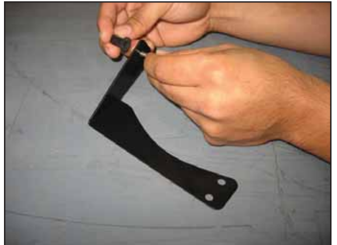
o. Fasten the supplied machine screw and wellnut to the bracket as shown. Hand tighten the machine screw into the wellnut.
