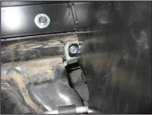
l. Install the supplied M6-1.0X20 bolt through the heatshield and the spacer. Thread it into the hole exposed in step 2q.
