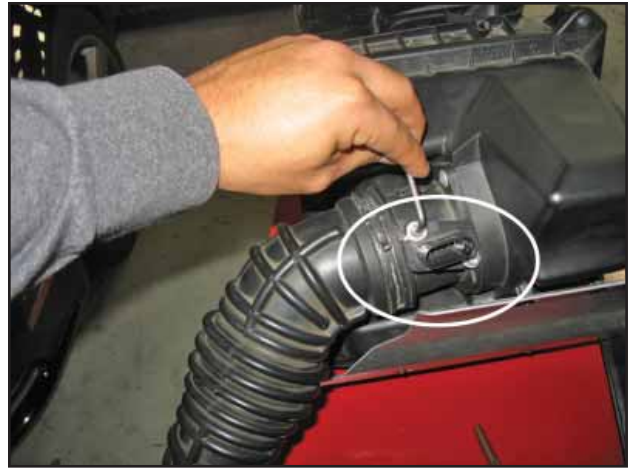
r. Carefully remove the MAF sensor from the stock housing using the supplied tamper-proof torx tool.
