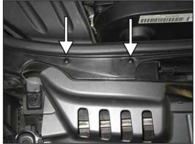
b. Remove the two screws located on the front of the fresh air duct.
