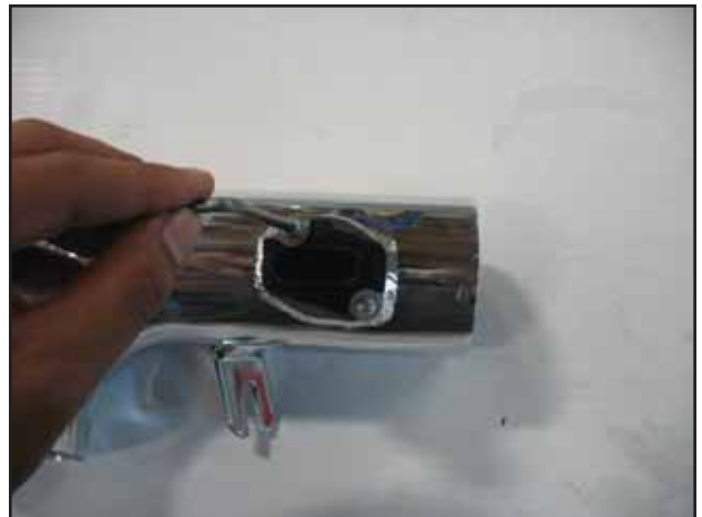
c. Insert the MAF sensor into the inlet pipe and secure with the stock screws.
