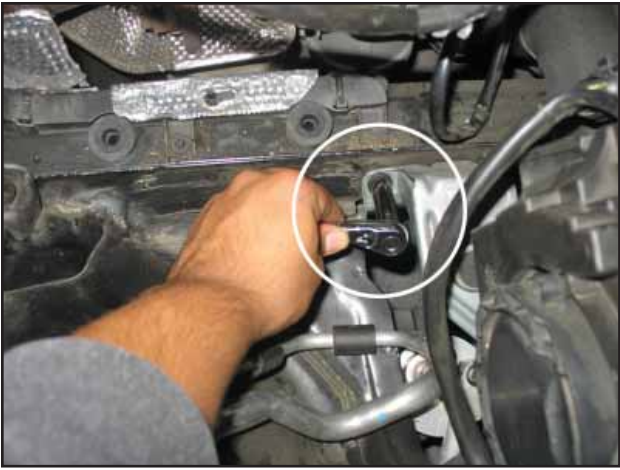
q. Remove the bolt securing the brace located beneath the passenger side headlight.
