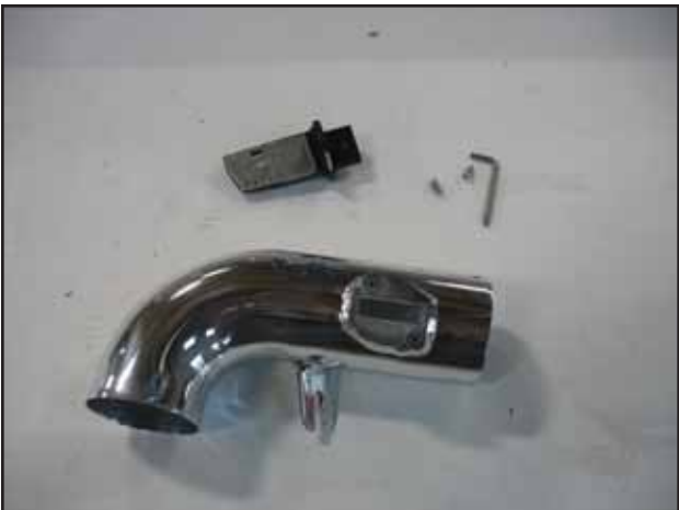
b. Use the stock MAF sensor screws and the supplied tamper-proof torx tool to secure the MAF sensor to the inlet pipe.
