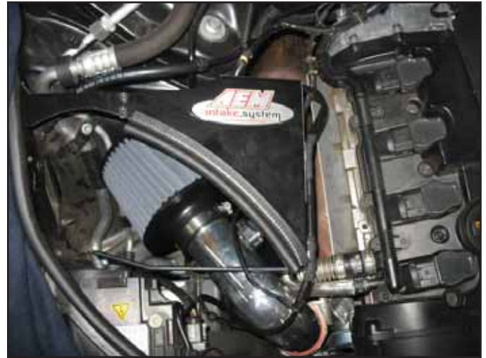
AEM® intake system installed
