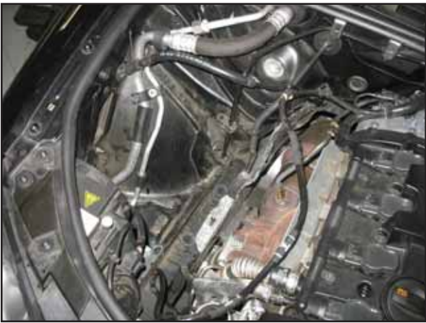
s. Factory air box system removed from the vehicle.
