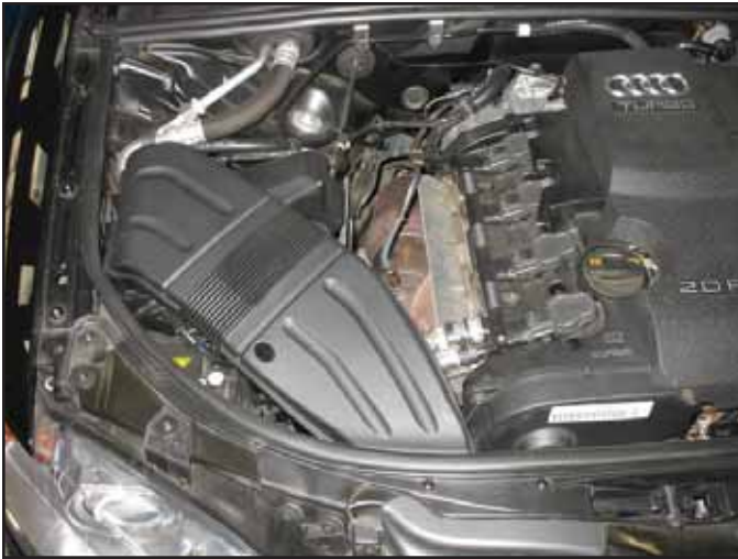
Factory air box system installed
