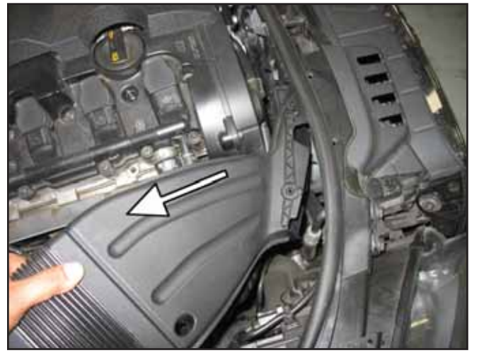
d. Slide the fresh air duct toward the firewall. Remove the fresh air duct from the fresh air scoop.
